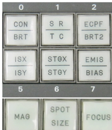
FIGURE 2. This is a selection of a few of the controls found on a typical SEM that uses a heated tungsten filament source. Terminology is often related to the control of the image rather than to the device in the accelerator being controlled. Changing some of the control names can help a student relate the control to the actual device and its operation in the accelerator system. For example, “Contrast & Brightness” (CON/BRT) can be “Detector Range & Gain”; “Magnification” (MAG) can be “Scanning Magnet Control”; “FOCUS” can be “Objective Magnet Control”; and “SPOT SIZE” can be “Condenser Magnet Control”.
