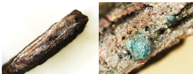
Fig. 1. Part of crucible wall No. Sz-656 with visible drops of alloy
