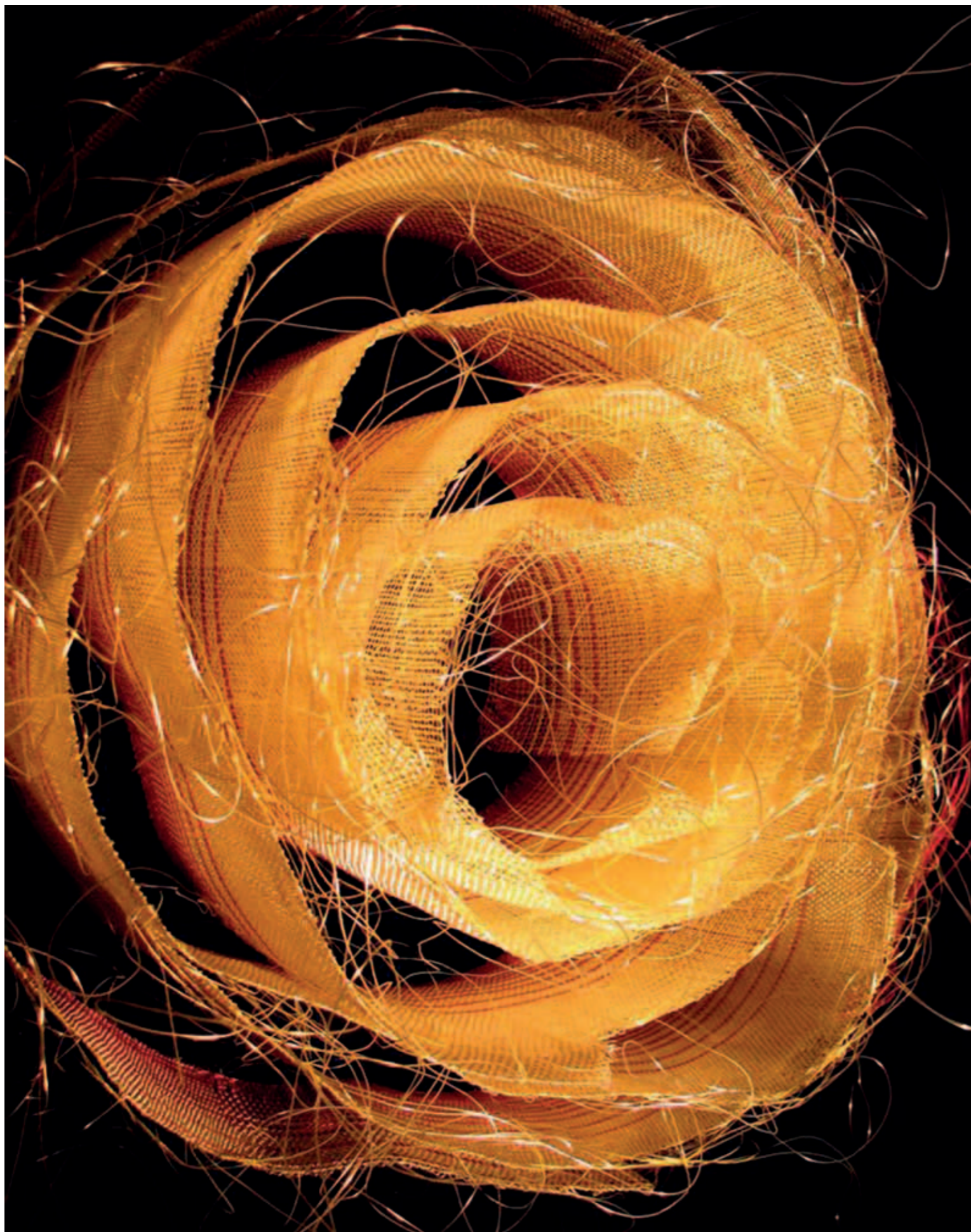
Textile Light Fitting. This reactive fabric is a combination of silver plated wire and luminescent yarn © Neil Musson MA RCA
