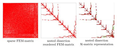
Fig. 3. Sparsity pattern of a 3D finite element matrix, its reordered finite element matrix according to nested dissection, and its corresponding H-matrix.
