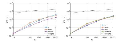
Fig. 9. Allocated storage per mesh degree of freedom for different admissibility conditions. Storage for nonsymmetric (left) and symmetric (right) matrices. The allocated storage is independent of the content of the matrix.
