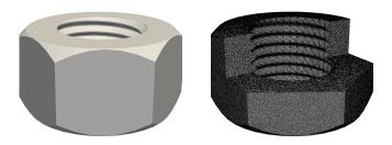
Fig. 10. The screw-nut geometry (left) and its meshed cross section (right).
