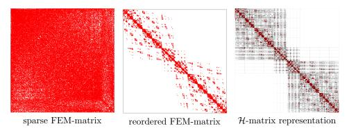
Fig. 1. Sparsity pattern of a 3D finite element matrix, its reordered finite element matrix, and the corresponding  $\mathcal{H}$ -matrix. Red blocks in the  $\mathcal{H}$ -matrix correspond to the nearfield, and white blocks correspond to the empty farfield.
