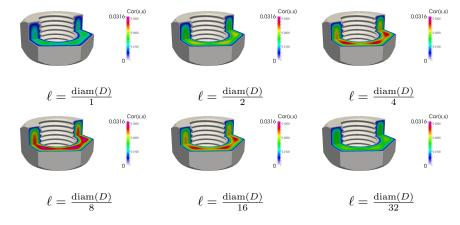
Fig. 12. Cross sections of the correlation of the solution through the screw-nut geometry for the Gaussian kernel with different correlation lengths  $\ell$ .
