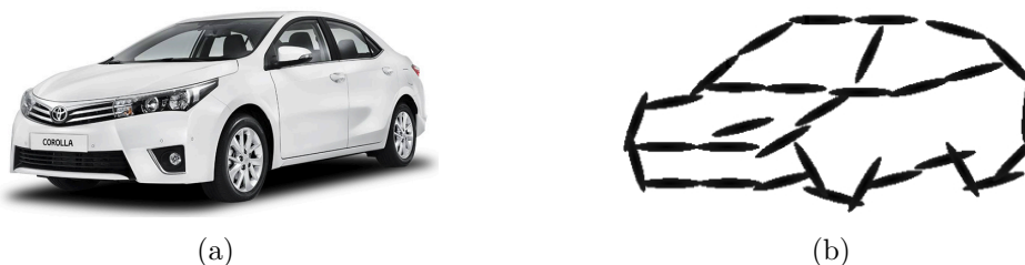
Figure 3.2: Schematic illustration of the basis decomposition result. (a) A training image. (b) Schematic illustration of the learned basis B_{\mathcal{R}} . Each of the ellipsoids represents a basis filter at a certain orientation and location. The overall shape of the basis template resembles the shape of the training image (adapted from [Wu et al., 2010]).
