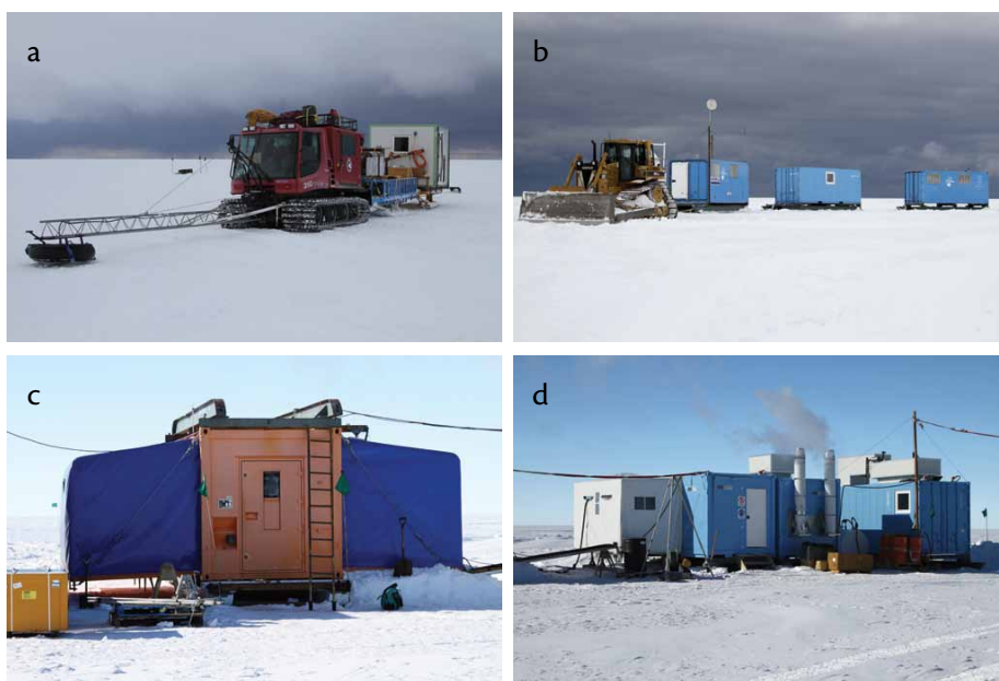
Figure 2. Traverse vehicles and ANDRILL hot water drill system (HWDS). (a) Pisten Bully with ice-penetrating radar boom deployed. (b) Caterpillar D6 bulldozer traversing ANDRILL camp and HWDS modules. (c) MECC (Mobile Expandable Container Configuration) with floor hatch and work area for instrument deployments through the ice shelf. (d) ANDRILL HWDS modules, including hose reel, hot water boilers and pumps, and generators.
