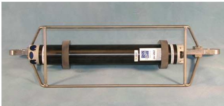
Figure 4: Nortek Aquadopp mounted on titanium load bar. No anti-fouling paint or transducer coating has been applied.
