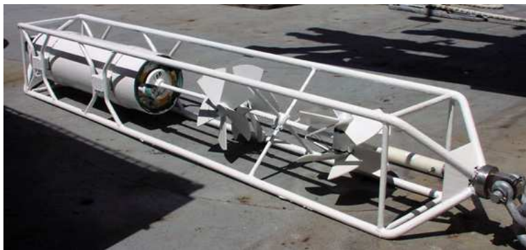
Figure 6: Vector Measuring Current Meter (VMCM) in mounted in stainless steel load cage. The cage, VMCM sting and VMCM pressure housing have been painted with a white anti-fouling coating.
