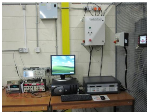
Fig.3. Dynamometer control and datalogging equipment
