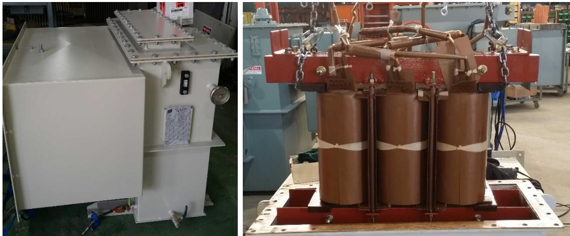
Figure 3.3 - Donated Earthing transformer from Excess Power Equipment for developing fault simulations.
