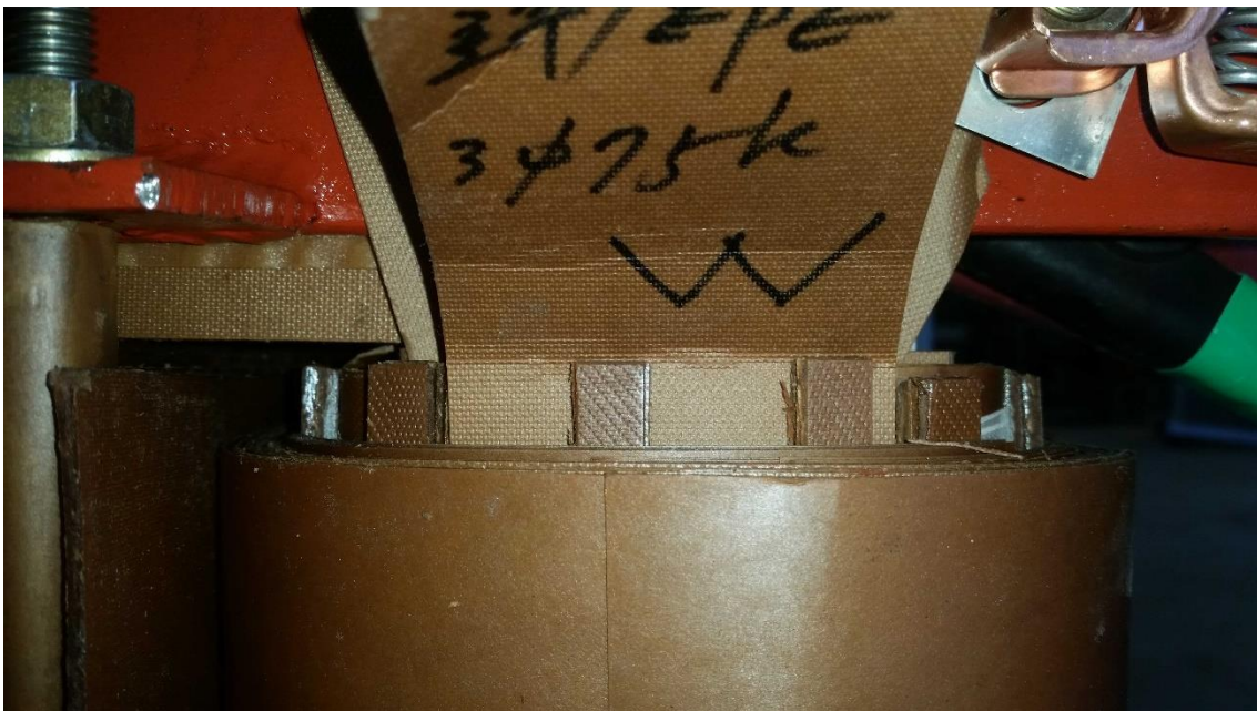
Figure 6.60 - North top view of 90% windings axial displacement test iteration.
