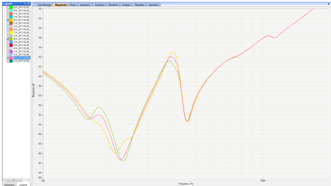
Figure 6.84 - Zoomed SFRA comparison results for short circuit testing
