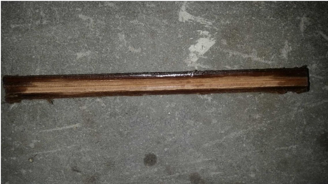
Figure 6.56 - Fabricated inner windings (inner core) spacer for 90% bulk windings movement test (Not in place as vantage point makes a photo un-recognisable)
