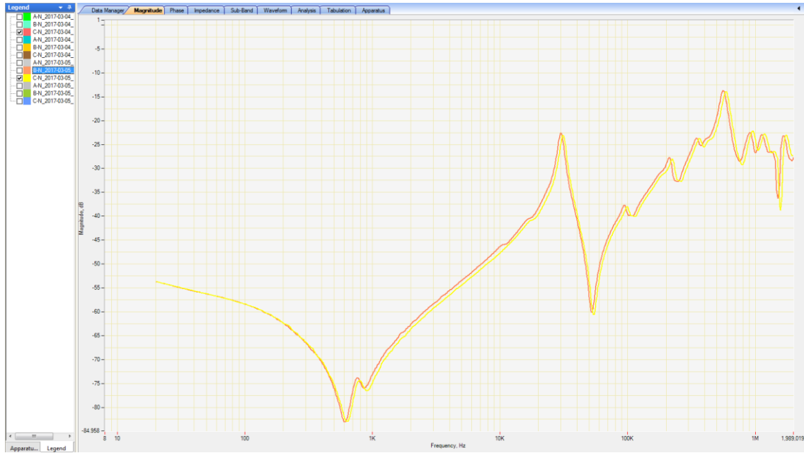
Figure 6.31 - SFRA comparison results for open circuit testing
