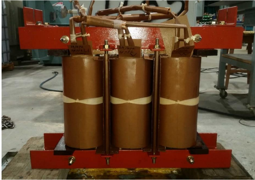
Figure 3.6 – Un-tanked earthing transformer core sitting on wooden blocks in an oil drip tray.
