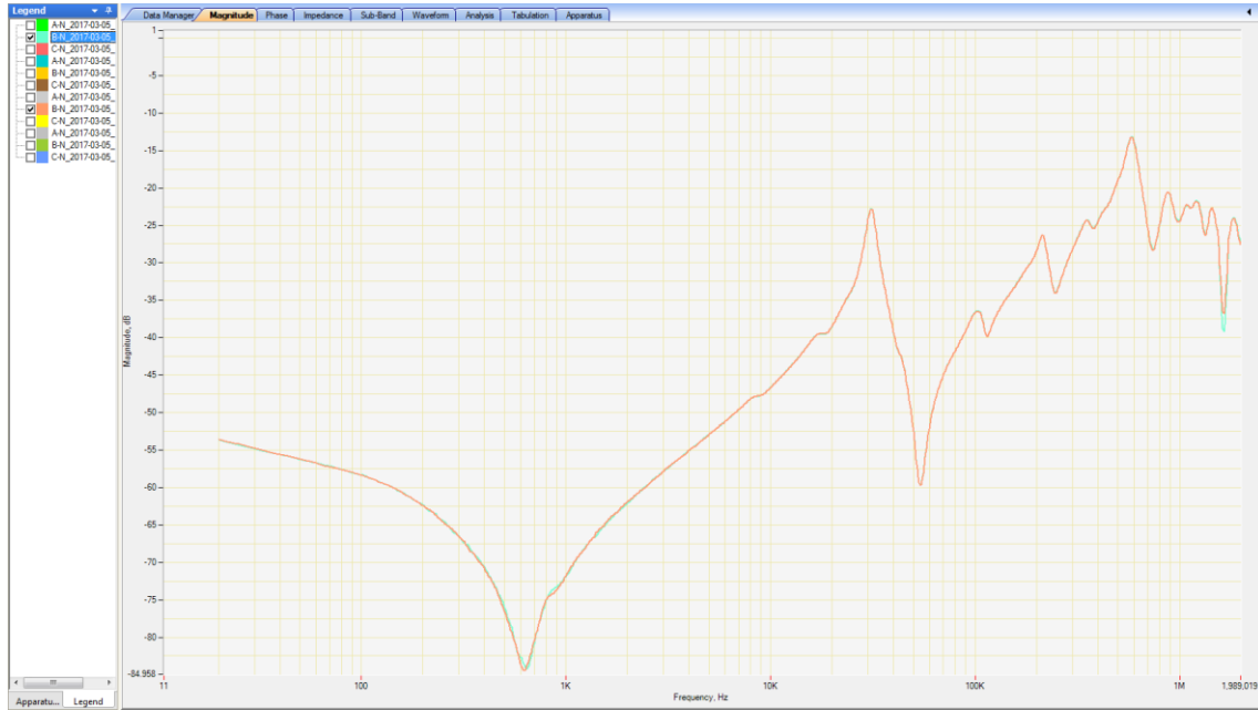
Figure 6.50 - SFRA comparison results for open circuit testing
