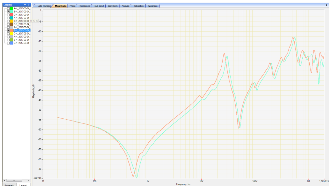
Figure 6.16 - SFRA comparison results for open circuit testing
