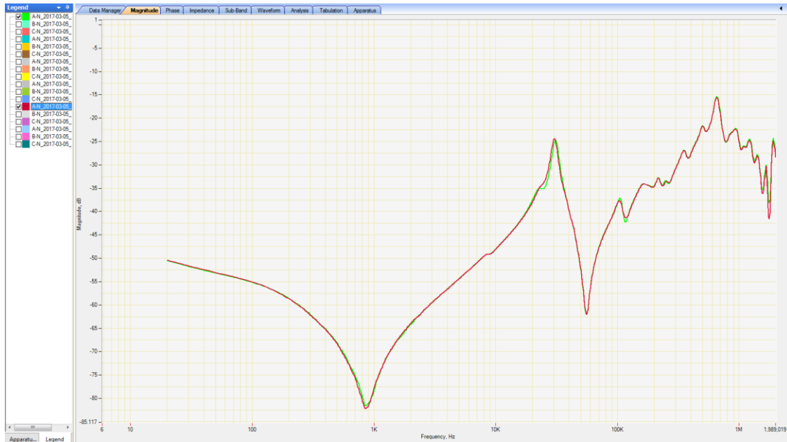
Figure 6.74 - SFRA comparison results for open circuit testing
