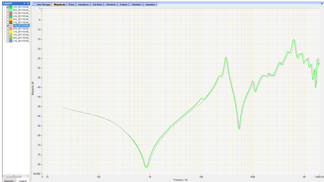
Figure 6.29 - SFRA comparison results for open circuit testing
