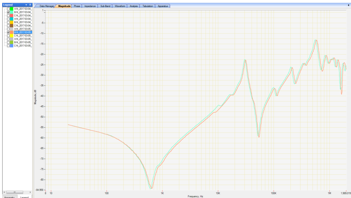
Figure 6.30 - SFRA comparison results for open circuit testing
