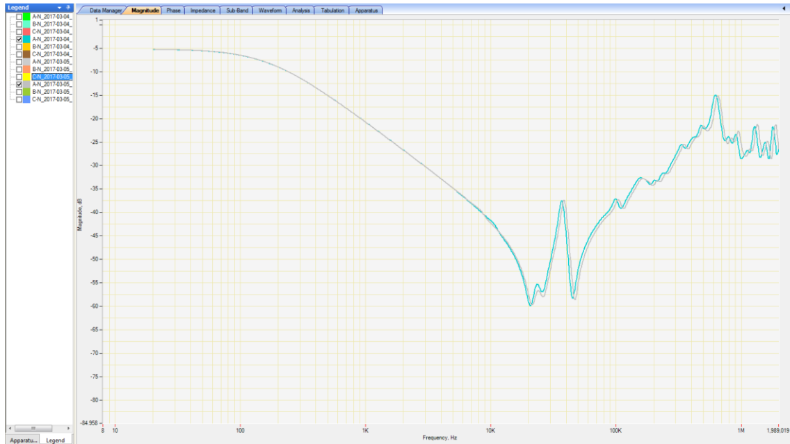
Figure 6.35 - SFRA comparison results for short circuit testing
