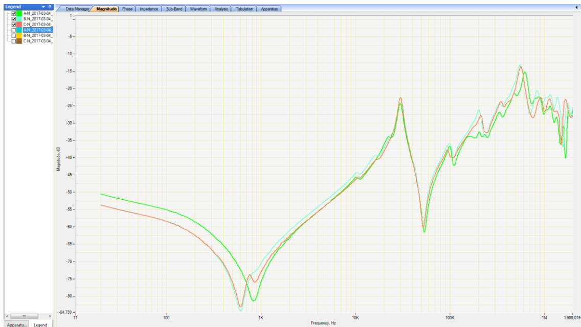
Figure 6.8 - SFRA phase comparison results for open circuit testing – Fully assembled
