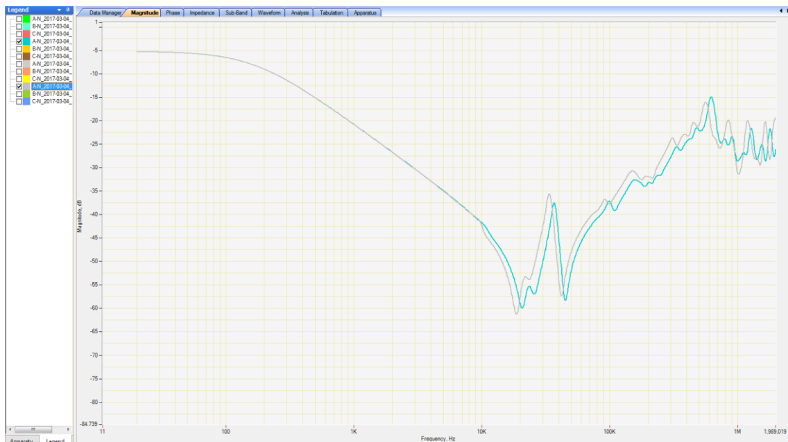
Figure 6.18 - SFRA comparison results for short circuit testing
