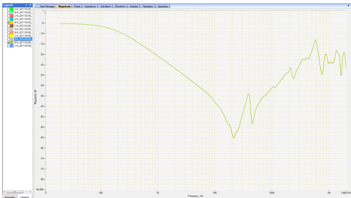
Figure 6.53 - SFRA comparison results for short circuit testing
