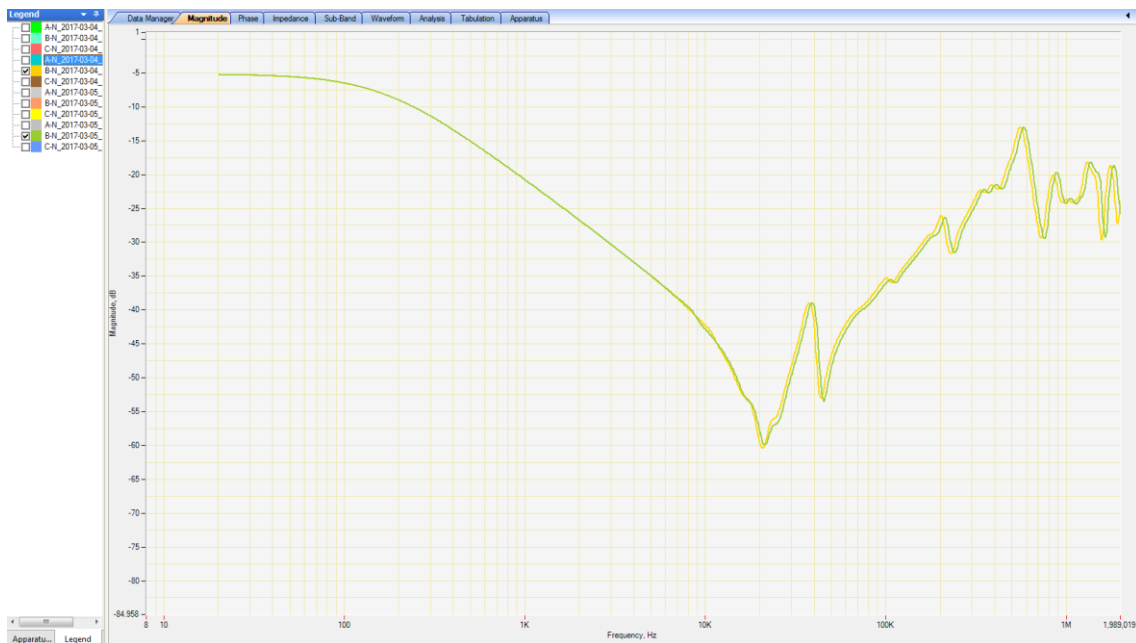
Figure 6.36 - SFRA comparison results for short circuit testing
