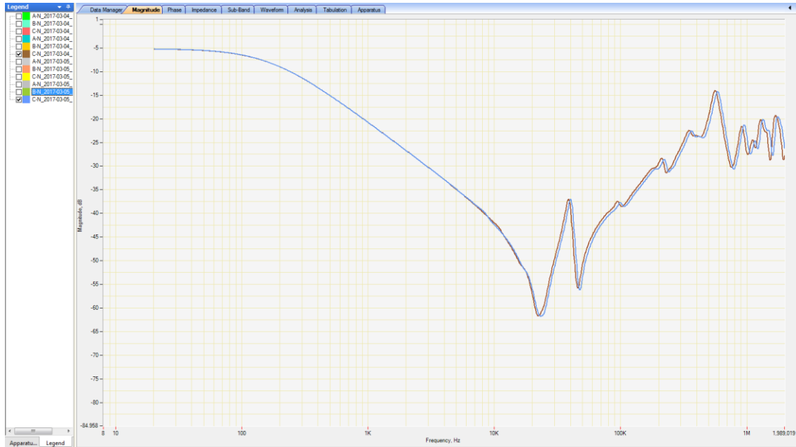
Figure 6.37 - SFRA comparison results for short circuit testing
