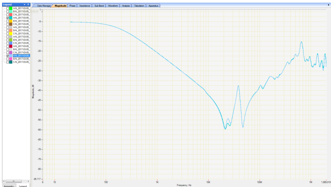
Figure 6.77 - SFRA comparison results for short circuit testing
