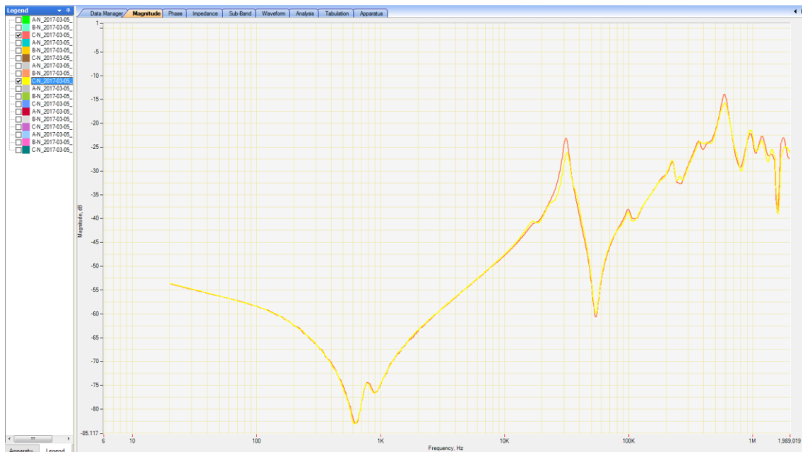
Figure 6.66 - SFRA comparison results for open circuit testing
