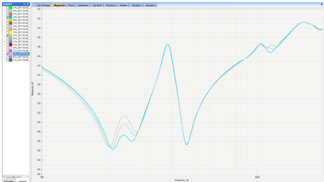
Figure 6.83 - Zoomed SFRA comparison results for short circuit testing
