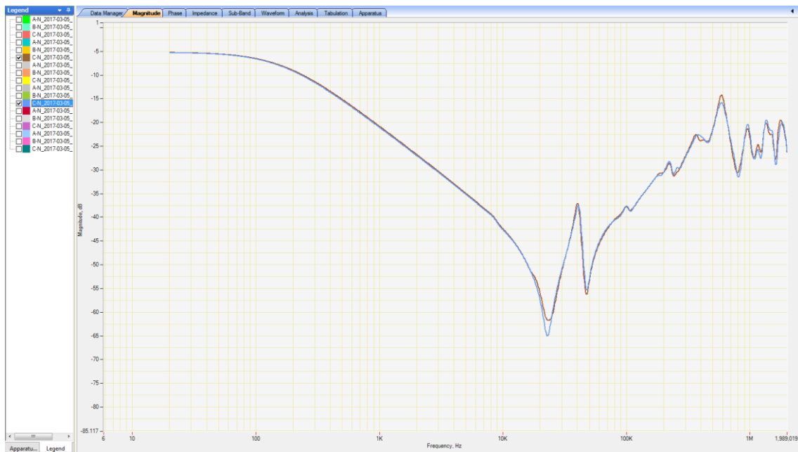
Figure 6.69 - SFRA comparison results for short circuit testing
