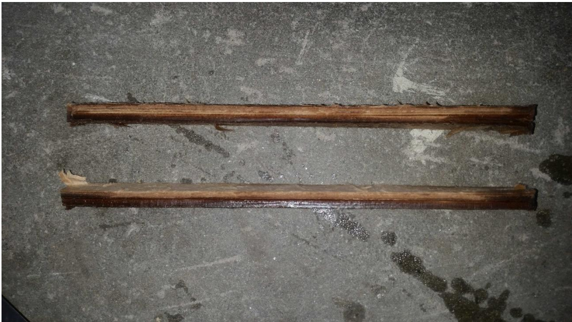
Figure 6.58 - Fabricated inner windings (inner core) spacer (made by splitting 90% spacer in half) for 45% bulk windings movement test (Not in place as vantage point makes a photo unrecognisable)
