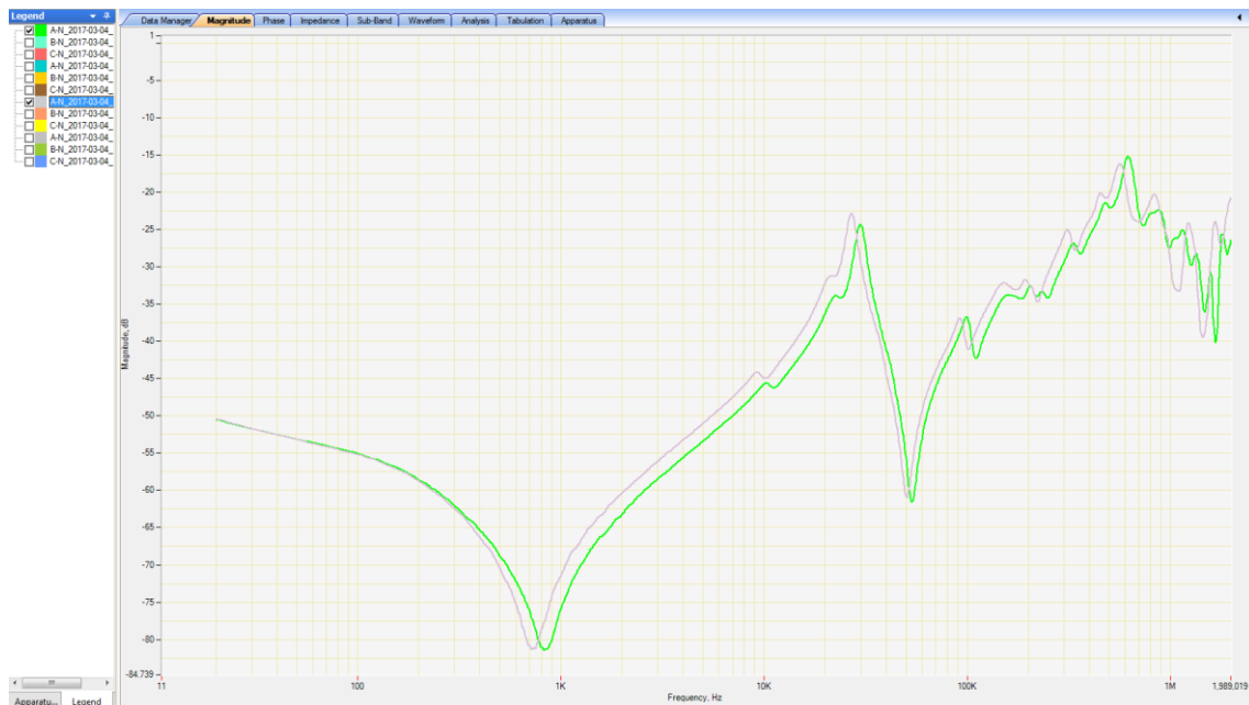
Figure 6.15 - SFRA comparison results for open circuit testing
