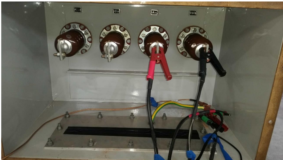
Figure 6.5 – Open circuit SFRA test set connection
