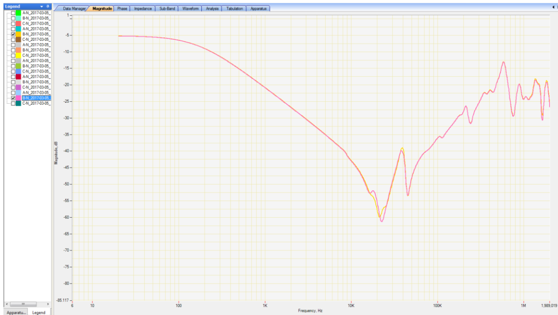
Figure 6.78 - SFRA comparison results for short circuit testing
