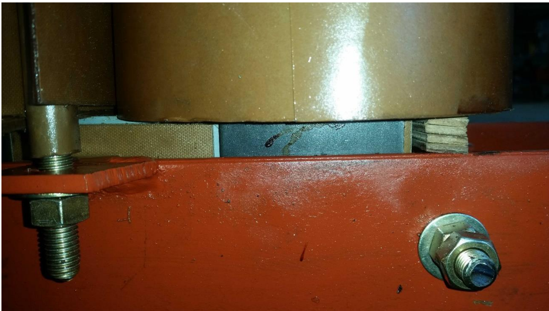
Figure 6.62 – North bottom view of 90% windings axial displacement test iteration.
