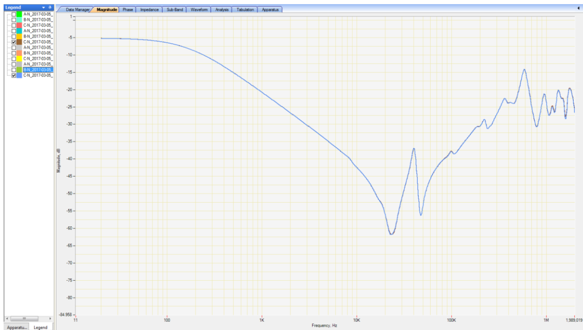
Figure 6.54 - SFRA comparison results for short circuit testing
