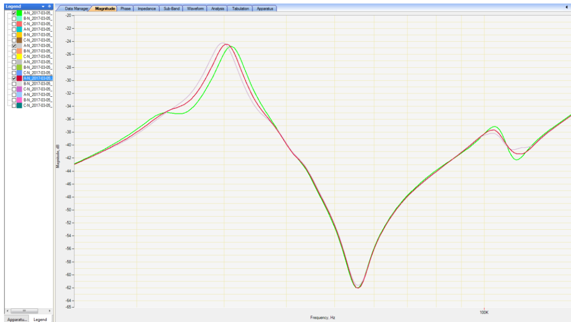
Figure 6.80 – Zoomed SFRA comparison results for open circuit testing
