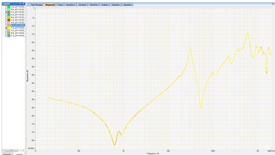
Figure 6.51 - SFRA comparison results for open circuit testing
