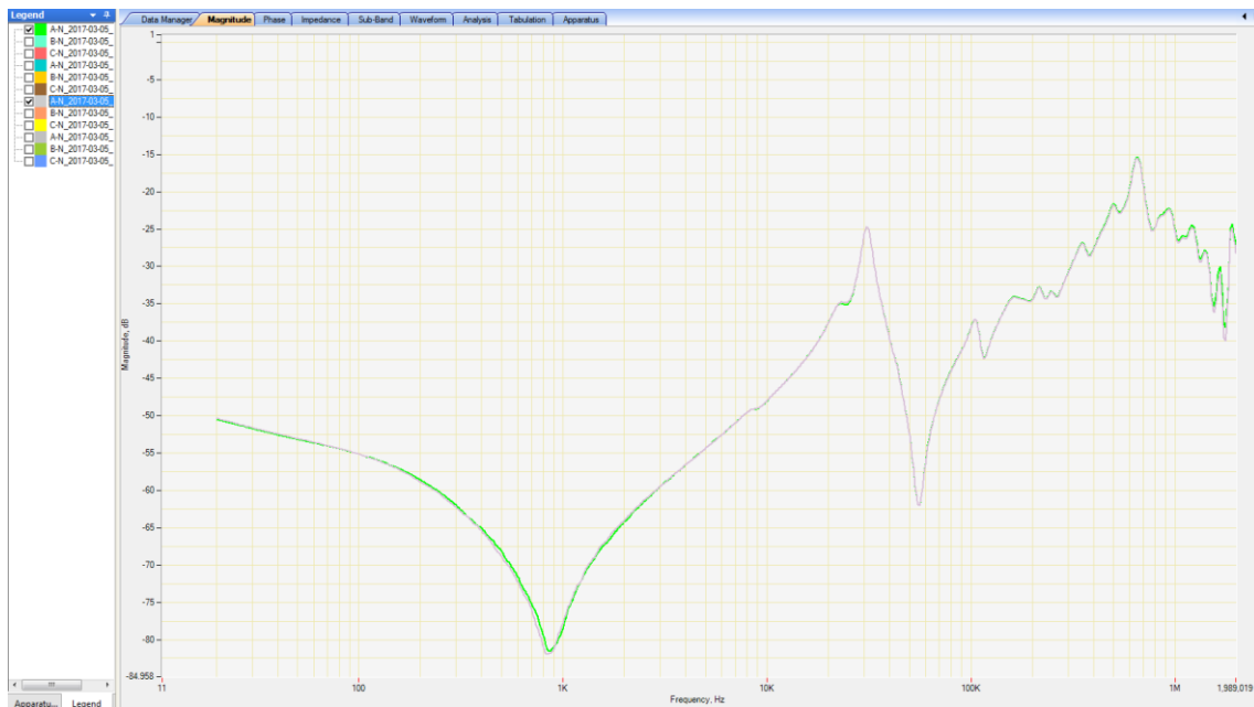
Figure 6.49 - SFRA comparison results for open circuit testing
