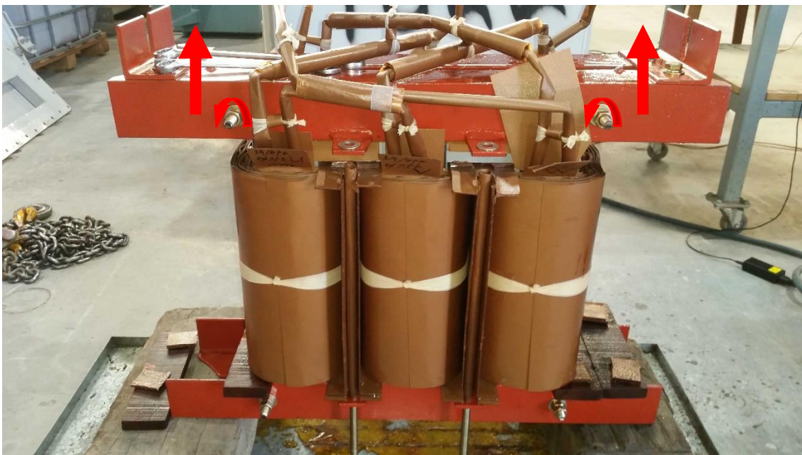
Figure 6.39 – Un-tanked transformer core and coils
