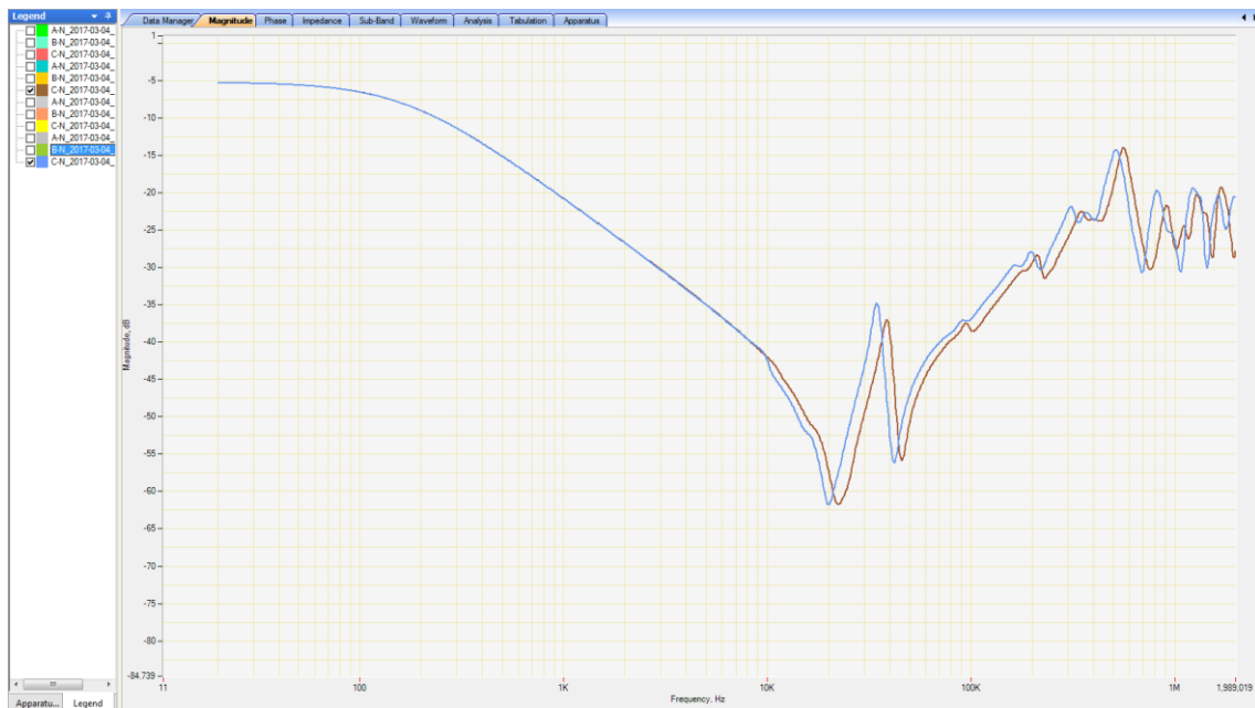
Figure 6.20 - SFRA comparison results for short circuit testing
