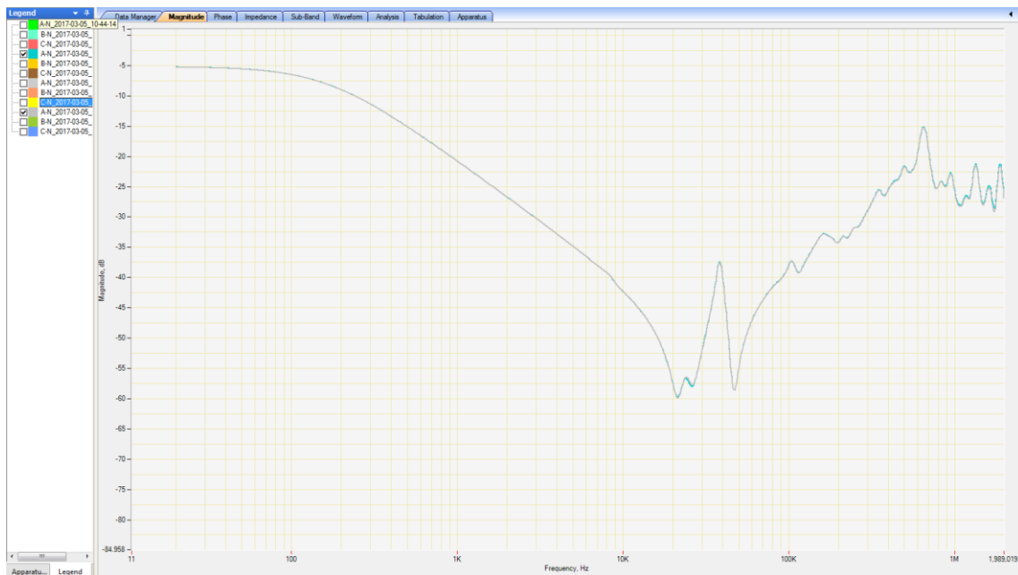
Figure 6.52 - SFRA comparison results for short circuit testing
