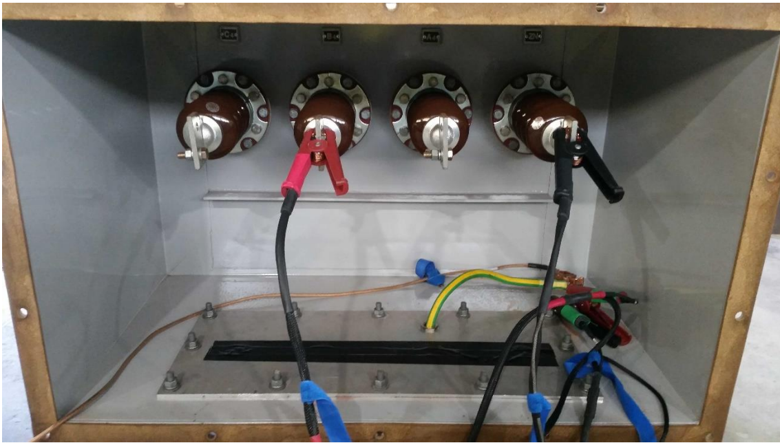
Figure 6.6 - Open circuit SFRA test set connection
