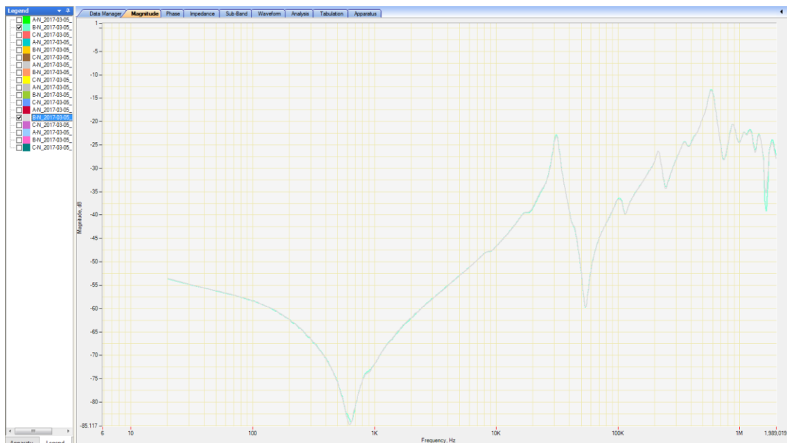
Figure 6.75 - SFRA comparison results for open circuit testing
