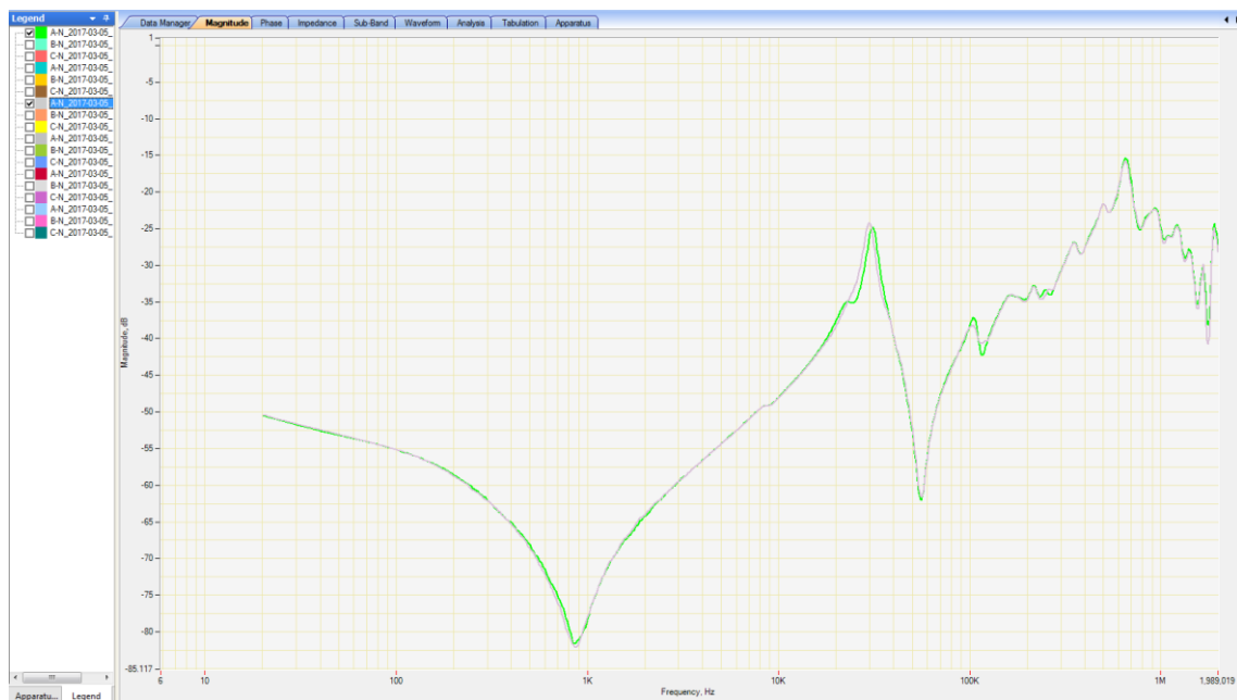
Figure 6.64 - SFRA comparison results for open circuit testing
