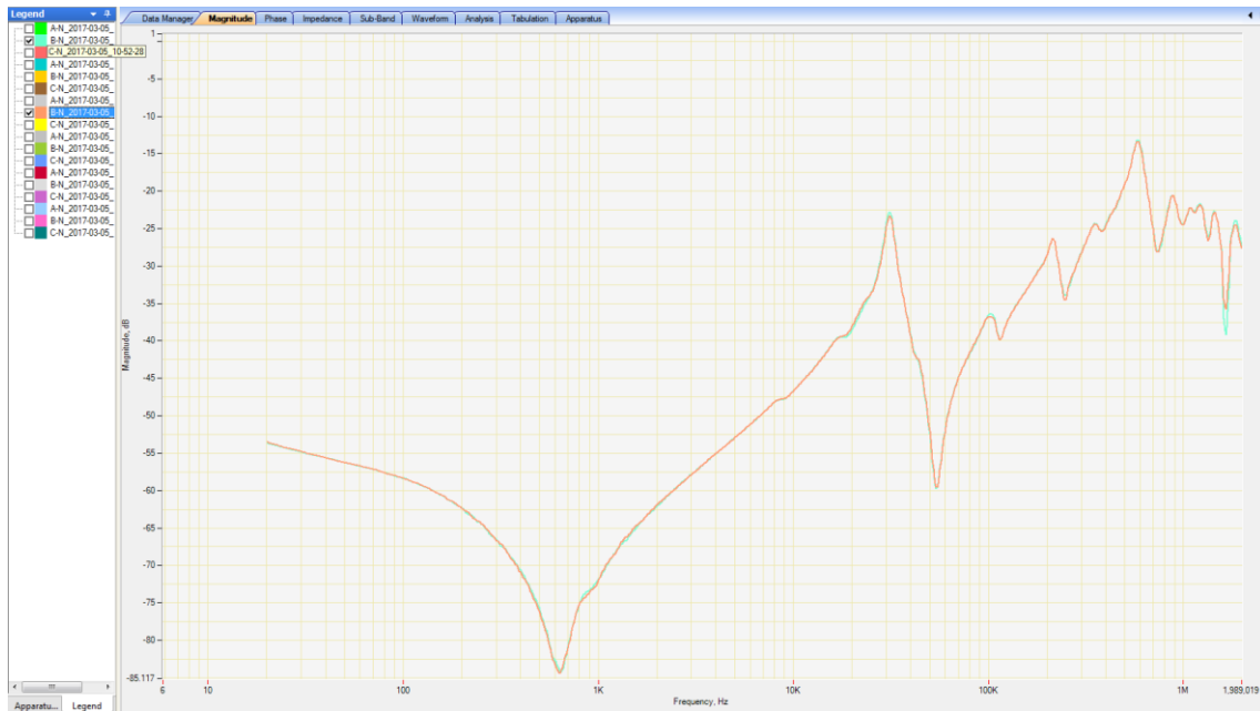
Figure 6.65 - SFRA comparison results for open circuit testing
