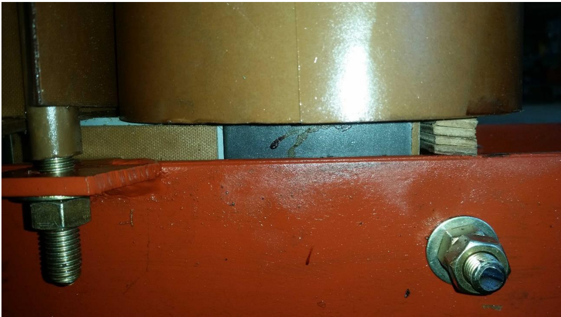
Figure 6.72 - North bottom view of 45% windings axial displacement test iteration.
