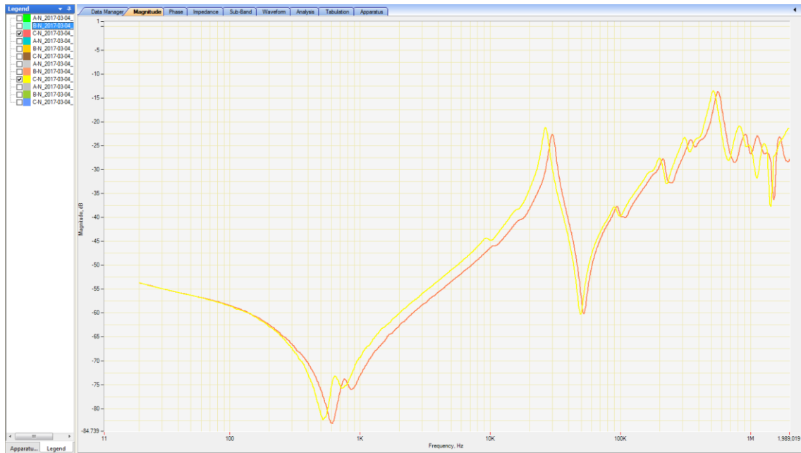
Figure 6.17 - SFRA comparison results for open circuit testing
