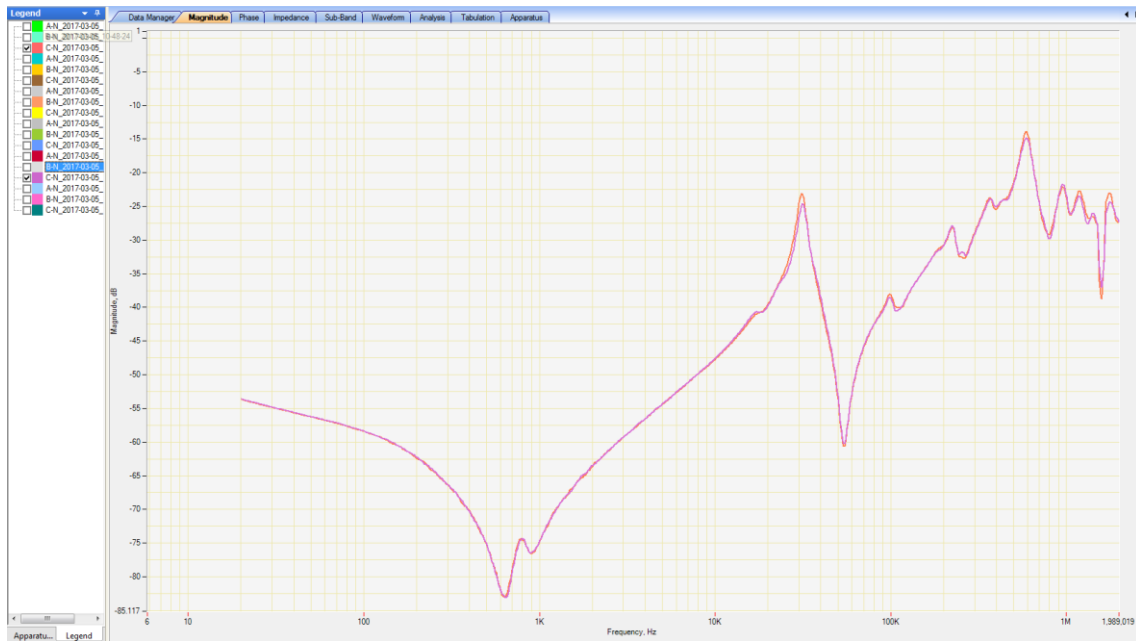
Figure 6.76 - SFRA comparison results for open circuit testing
