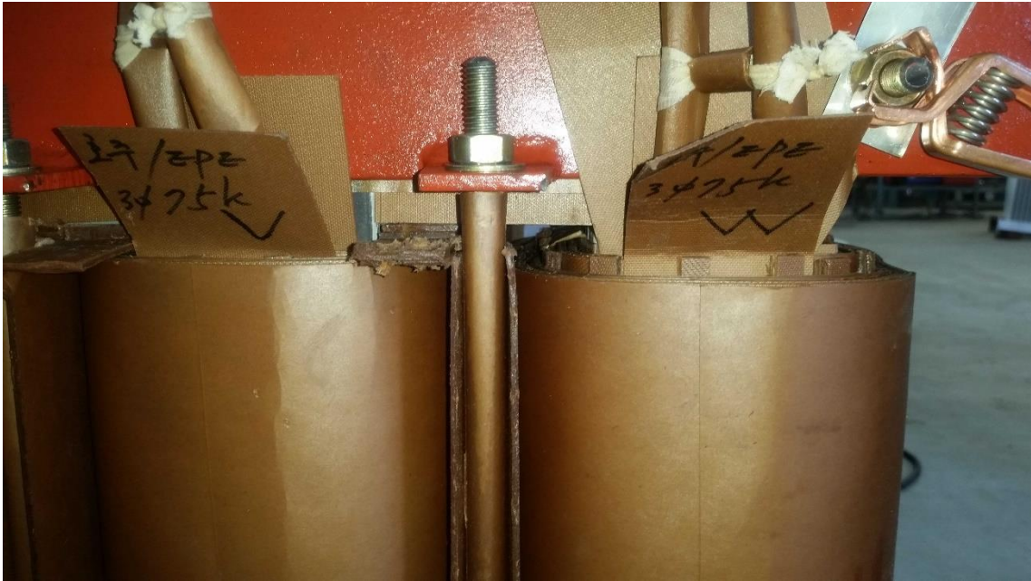
Figure 6.70 - North top view of 45% windings axial displacement test iteration.
