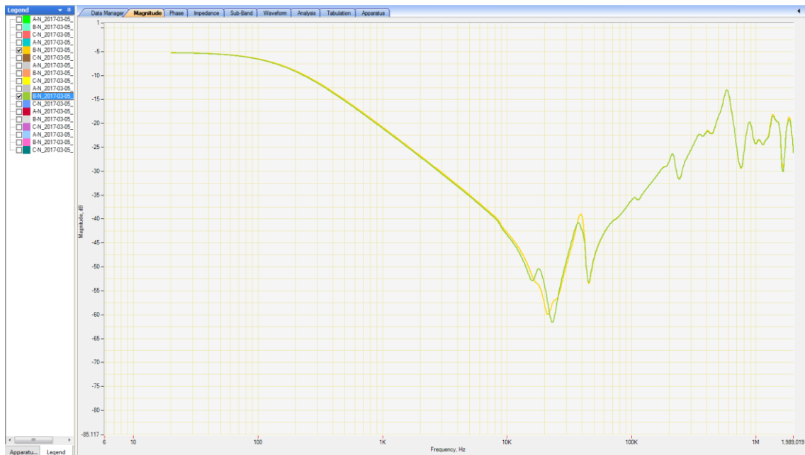
Figure 6.68 - SFRA comparison results for short circuit testing
