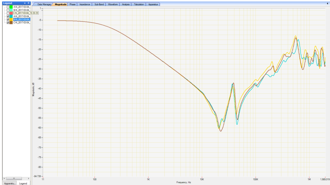
Figure 6.12 - SFRA phase comparison results for short circuit testing – Fully assembled
