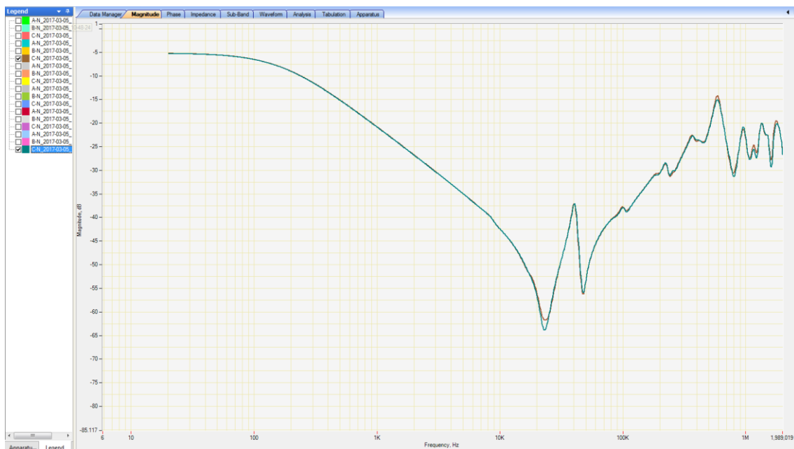
Figure 6.79 - SFRA comparison results for short circuit testing
