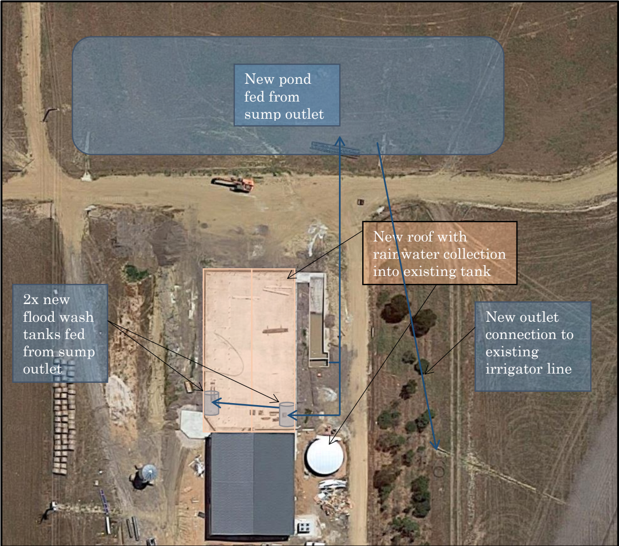
FIGURE 24 - FINAL OVERALL SITE LAYOUT
