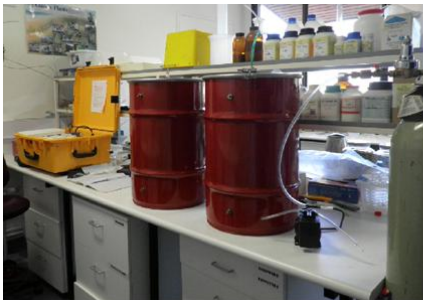
Figure 2 The fumigation chamber (47.8 cm x 40.6 cm internal diameter) equipped with gas injection and sampling systems.
