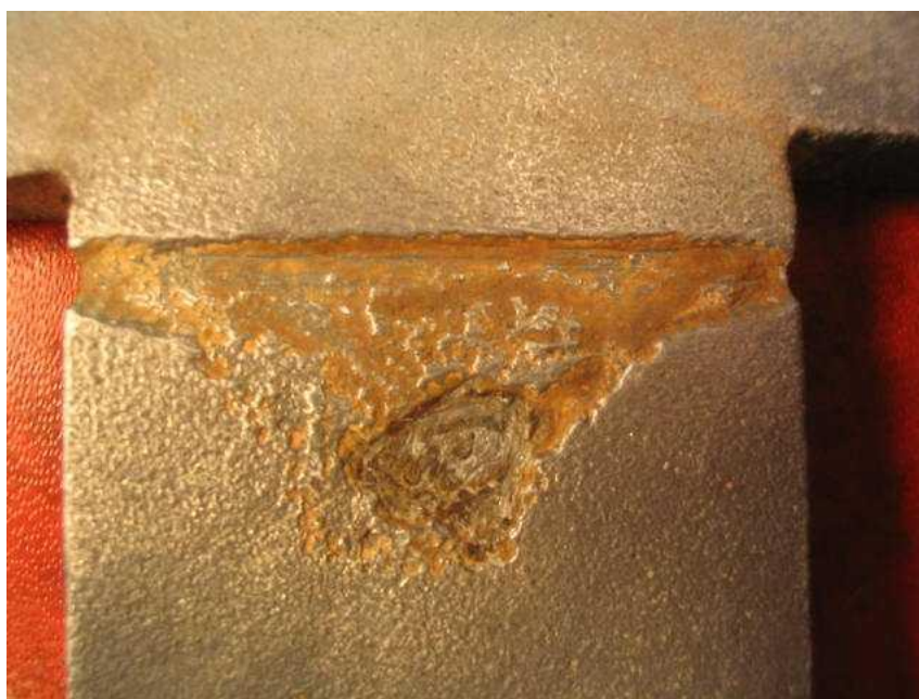
Fig. 12. Corrosion of a Pb-Ag anode close to the solution line
