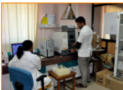
Trace metal analysis in Atomic Absorption Spectrophotometer
