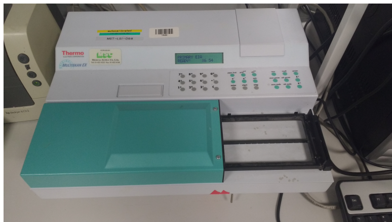
Figure 2.5: Photograph of the Multiskan Ex Photometer used in all ELISA experiments
