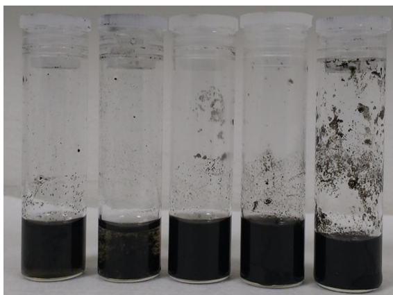
Figure 2.34: MWCNT solutions at concentrations of 0.05, 0.1, 0.3, 0.5 and 1 mg/ml (left to right) in 1:1 water/DMF
