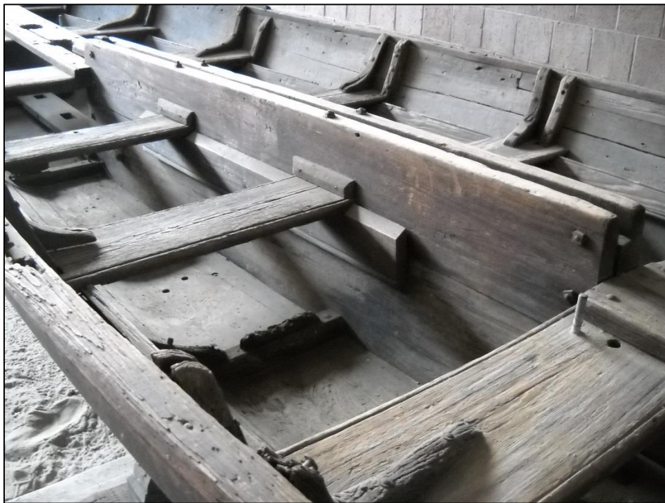
Figure 38: Centerboard Trunk and Surrounding Structure looking forward from Port Side (photo by ECU Fall Field School 2010)
