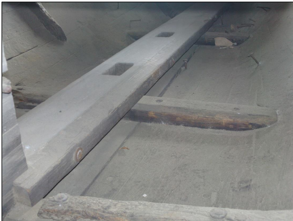
Figure 36: Forward Mast Steps and Floor Timbers from Starboard Side (photo by author 2012)
