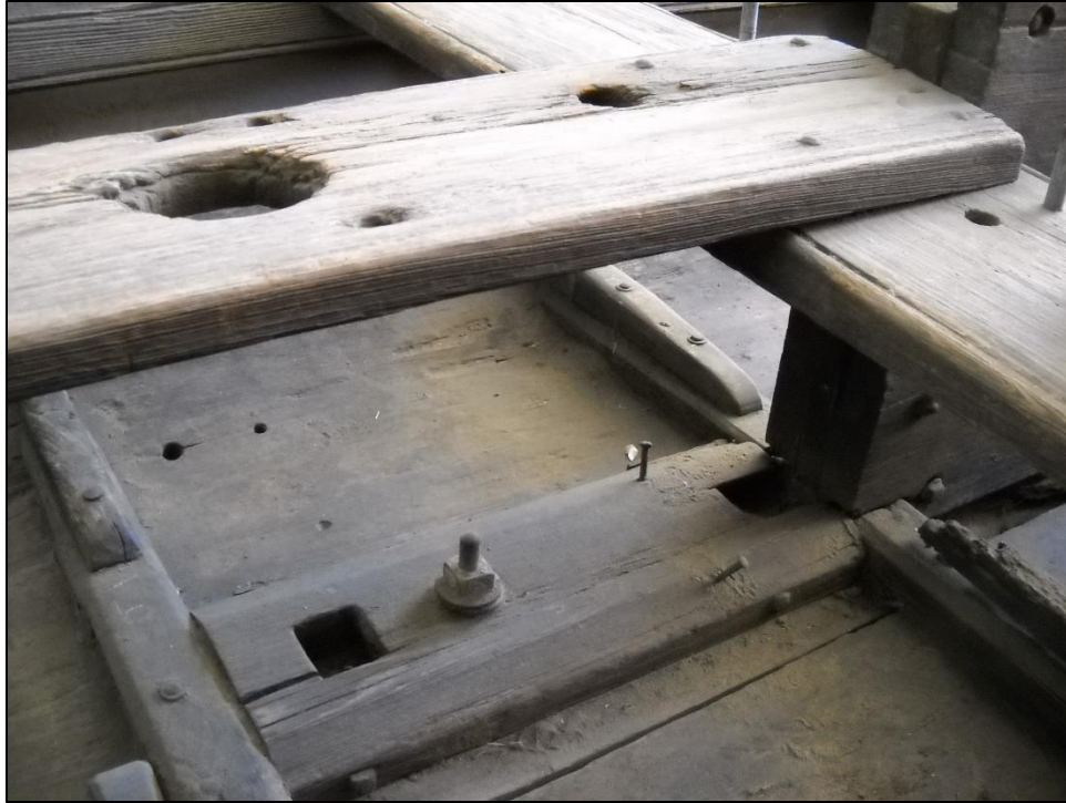
Figure 37: Aft Mast Steps and Partner from Starboard Side (photo by ECU Fall Field School 2010)
