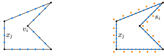
Figure 5.2. Nodes used by BEM (left) and nodes and sites used by MFS (right).
