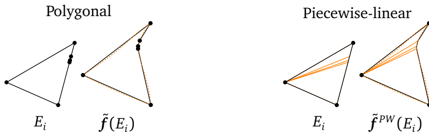
Figure 10.2. Comparison of f (orange dashed line) with its polygonal \tilde{f} and piecewise-linear approximations \tilde{f}^{PW} (black solid line) for an element E_i .
