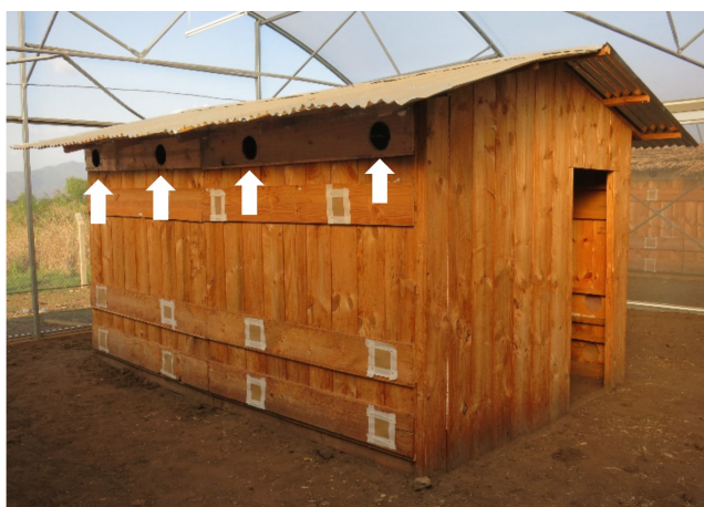
Figure 2. Semi-field experimental wooden hut used for the video surveillance experiments in a screen house in Kining'ina, Ifakara, Tanzania. Eave tubes are indicated by white arrows.
