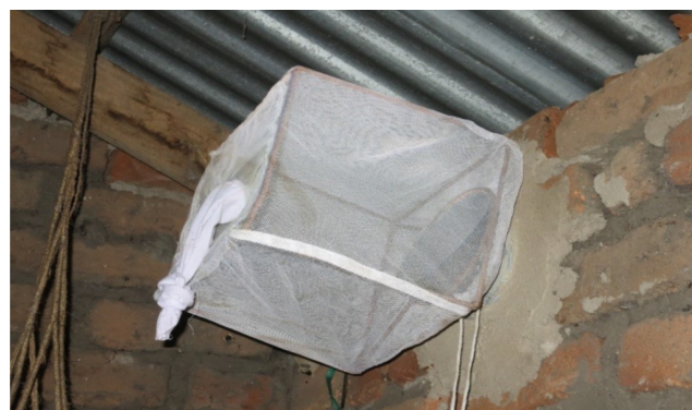
Figure 6. Eave tube entrance trap mounted on an eave tube in a house in Sagamaganga. The white net treated with Ficam W® to ensure rapid knockdown upon contact.
