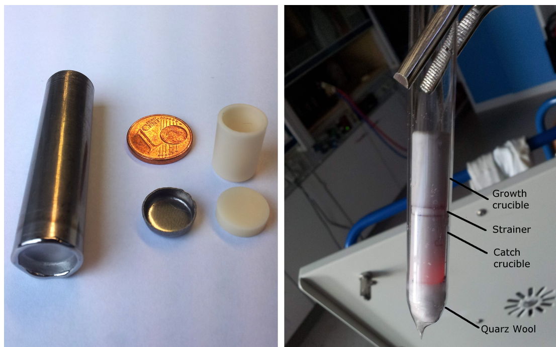
FIGURE 3.4: (Left) Niobium and alumina crucibles with caps for high-temperature synthesis of the \text{Eu}(\text{Fe}_{1-x}\text{Ru}_x)_2\text{As}_2 series. (Right) Quartz-tube assembly directly after separating the liquid flux from the \text{Eu}_{1-x}\text{Ba}_x\text{Fe}_2\text{As}_2 crystals into the catch crucible (bottom) through a strainer (middle) from the growth crucible (top) via centrifuging at around 750 rpm for a few seconds. The glowing flux is still visible at the bottom.
