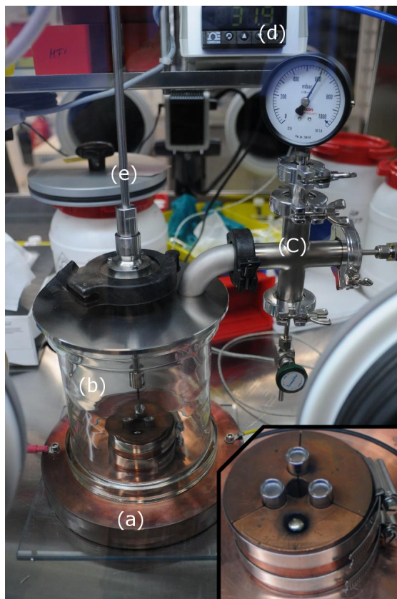
FIGURE 3.2: New in-box arc melter, with (a) copper base, (b) glass recipient, (c) vacuum tubing, and (d) thermocouple to monitor the temperature of the Cu block during welding. The electrode (e) can be moved freely within the entire glass recipient and, in particular, allows for sealing crucibles of varying height. The inset shows a magnification of the improved sample holder, which can now accommodate four samples (three shown) and features a depression for the oxygen getter—a piece of Zr.
