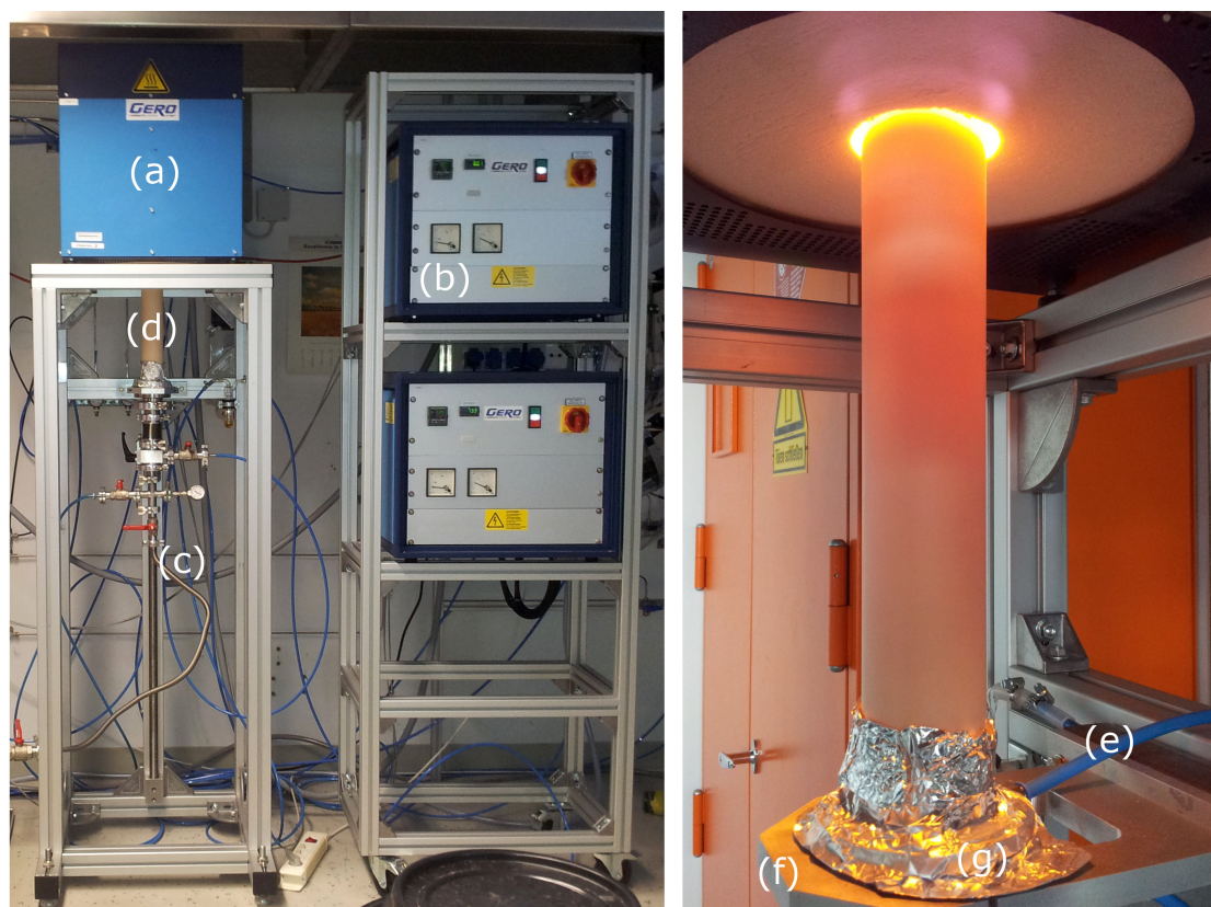
FIGURE 3.1: (Left) High-temperature furnace assembly with (a) commercial heating unit, (b) power supply unit, (c) vacuum tubing, and (d) sealed growth chamber. (Right) Sealed furnace chamber during growth at 1500 °C with (e) water cooled (f) metal flange covered by (g) a radiation shield made of Al foil to protect the adhesive bond between the flange and the \text{Al}_2\text{O}_3 .
