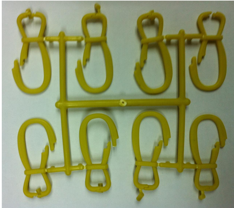
Figure 3. A photo of a test shot produced by a “One Product Mould” ( Courtesy: the supporting company )
