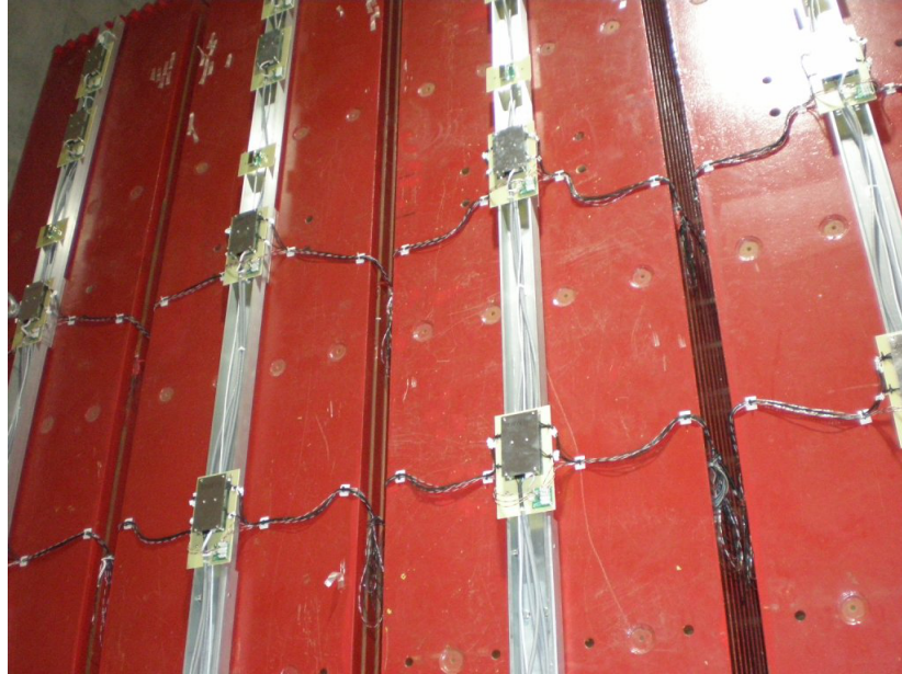
Figure 2.24: A photograph of some SMRD modules positioned between the magnet return yokes. The readout boards can be seen positioned with each of the modules. Photograph taken from [67].
