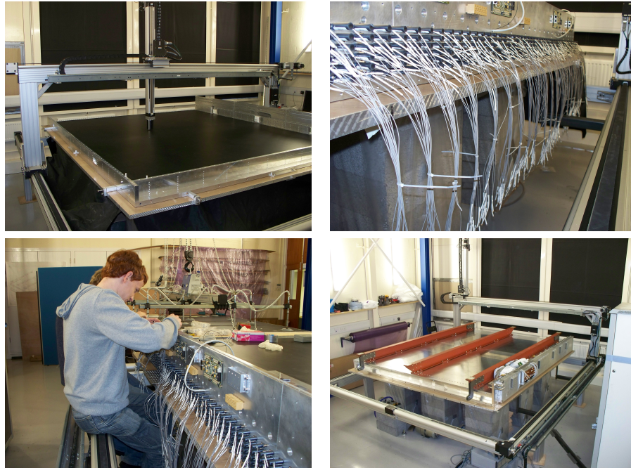
Figure 2.23: Top left: The scanner used to check for fibres damaged in the insertion process. Top Right: All MPPCs connected to the fibres and mounted on the bulkhead. Bottom Left: Connection of the coaxial cables from the MPPCs to the front-end electronics. Bottom Right: The finished P0DECal left side module.
