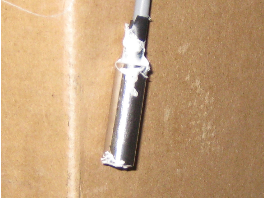
Figure 6.11: One of the digital thermometers on the outside of the tank, inside its protective casing.
