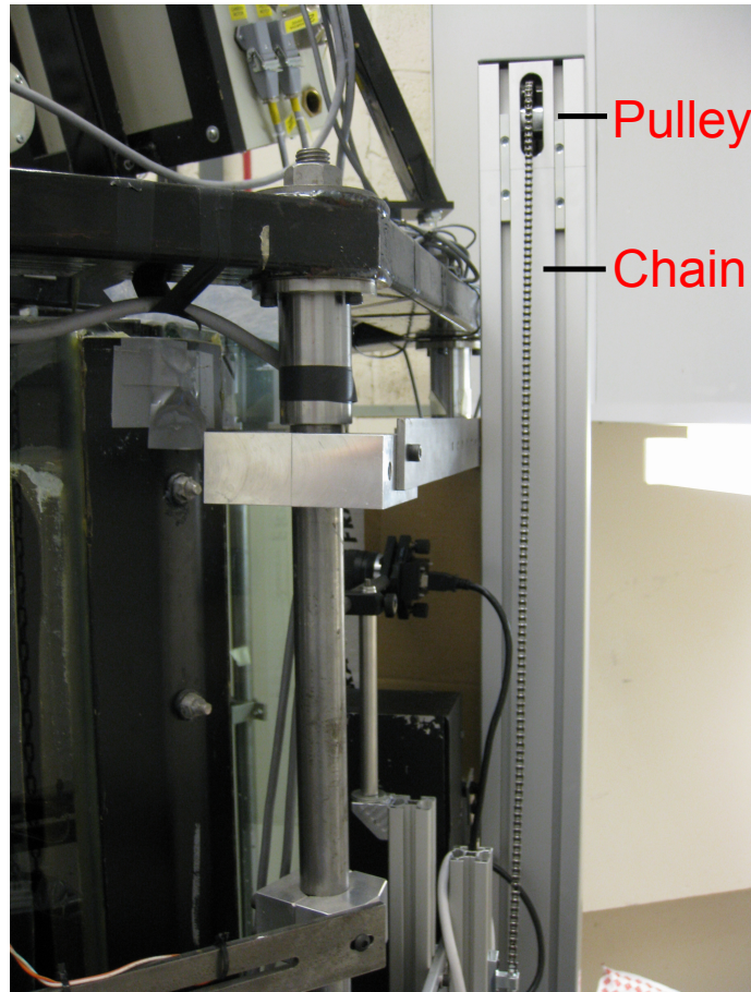
Figure 6.10: The chain and pulley system connects the traverse to the counterweights moving inside the vertical members.
