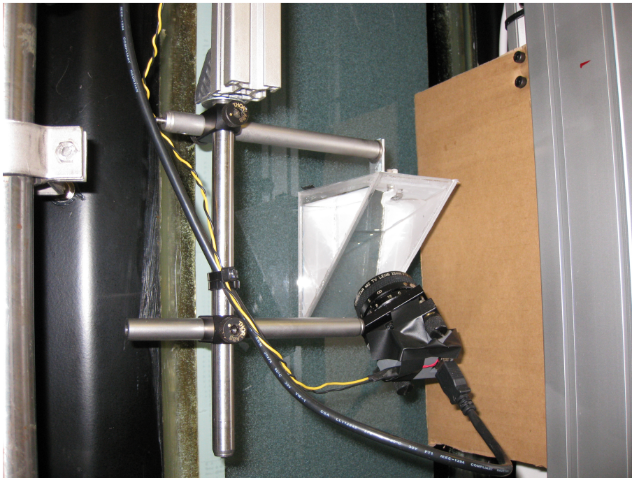
Figure 7.10: Perspex water filled refractive index matching prisms
