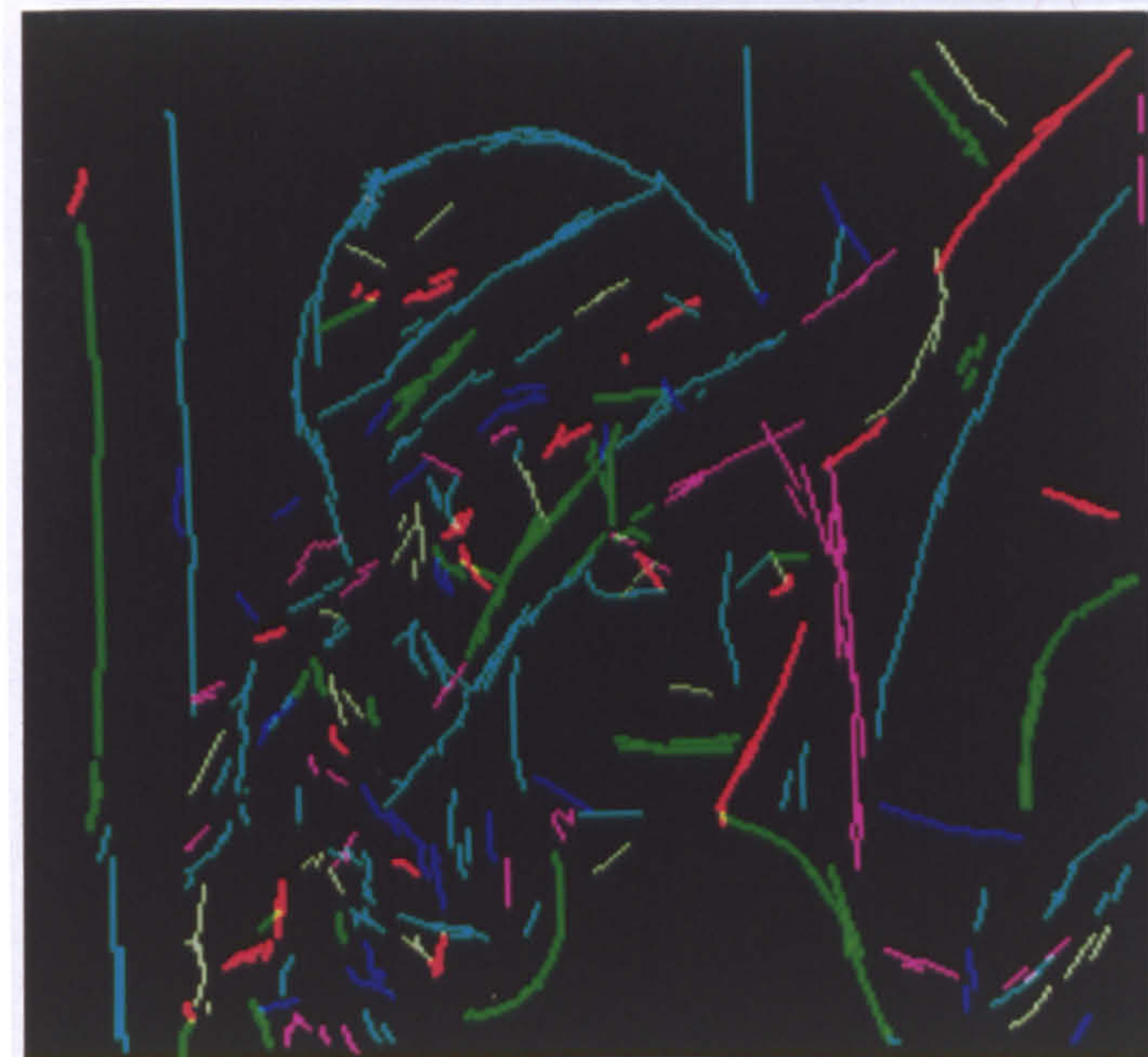
Figure 5.18: Lena: Feature linking - with backtracking for missed features.
