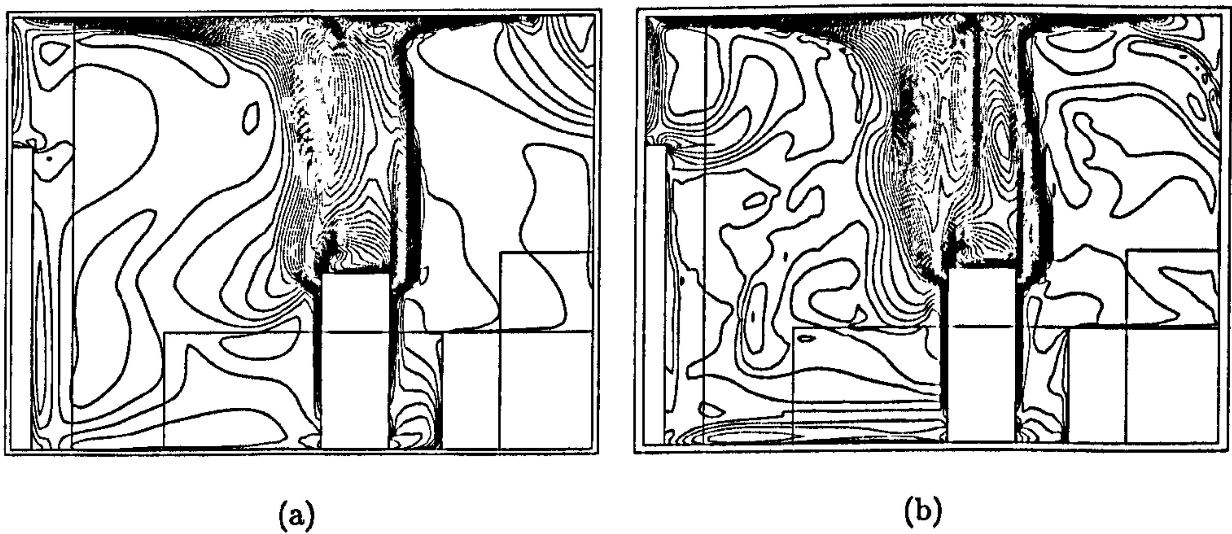
Figure 11.7: Velocity contour plots in the DIN man's mid-plane for Case 06. (a) linear and (b) EASM k - \epsilon model.
