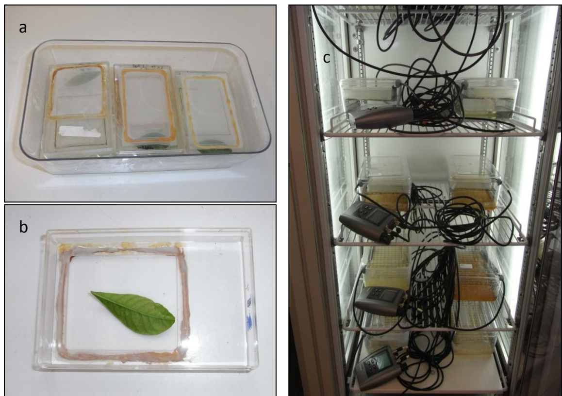
Figure 3.2: a) Experiment arena containing a C. ternata leaf infested with T. urticae eggs; b) Box containing arenas and salt solution to maintain humidity; c) Controlled environment cabinet containing boxes and data loggers.
