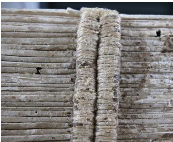
Detall nervis , cosit monacal compensat
