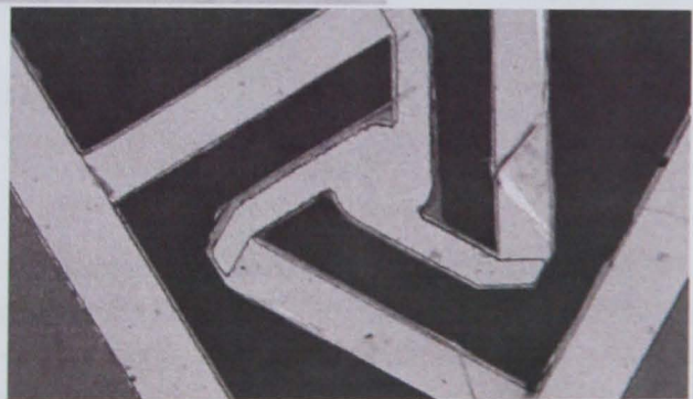
Figure 6.23: Fabrication defects on artefact A, obtained using a digital optical microscope.
