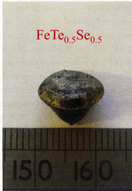
Figure 3.2: A sample of \text{FeTe}_{0.5}\text{Se}_{0.5} , made by the two-step self-flux method.
