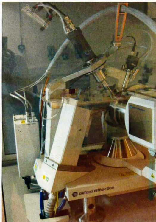
Figure 2.4: An Oxford Diffraction CCD single crystal diffractometer. The figure shows the sample on a four-circle goniometer, the cryo-jet, X-ray source, CCD and beam stop.
