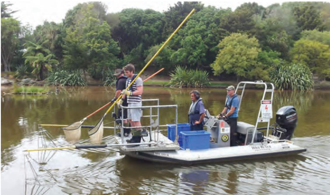
PLATE 4.10 The 4.5 m long, aluminium-hulled electrofishing boat developed by The University of Waikato in 2003, showing the anode poles at the bow, the generator at stern positioned under the boat driver's seat, and fibreglass-handled dip nets for retrieving fish.
