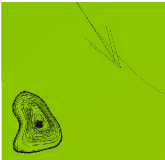
Fig. 7. Enlarged view of the separated flow in the corner region.
