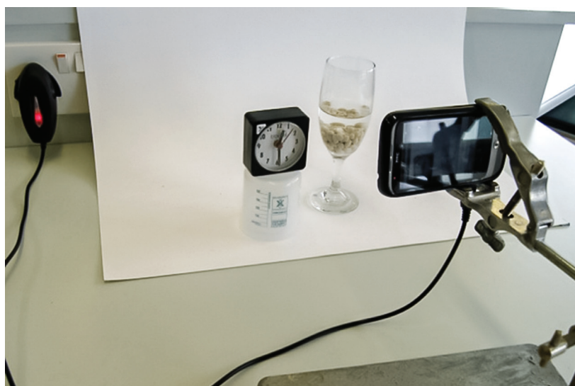
Figure 2 The laboratory set-up for recording a time-lapse movie
