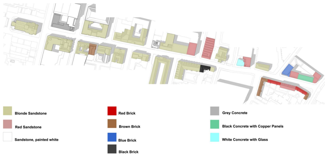
Figure 2 - Ingram Street Cladding Materials
