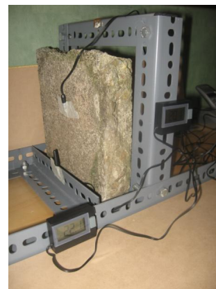
Figure 4 - Thermometers T2 and T3 in place
