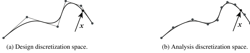
Fig. 6. Two levels NURBS discretizations: (a) Coarse discretization for design, (b) Refined discretization for analysis.
