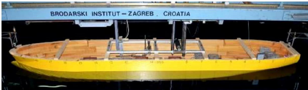
Fig. 2 Towing tank experiment with tanker model [20]
