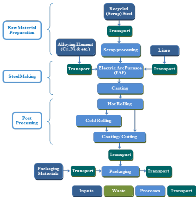
Figure 2: Process map of stainless steel manufacturing
