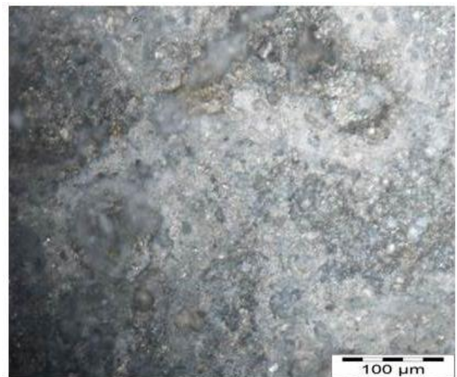
Figure 4: Morphology of Zn-40ZnO-1.0 A composite coating
