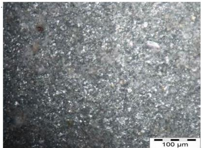
Figure 2: Morphology of Zn-20ZnO-1.0A composite coating
