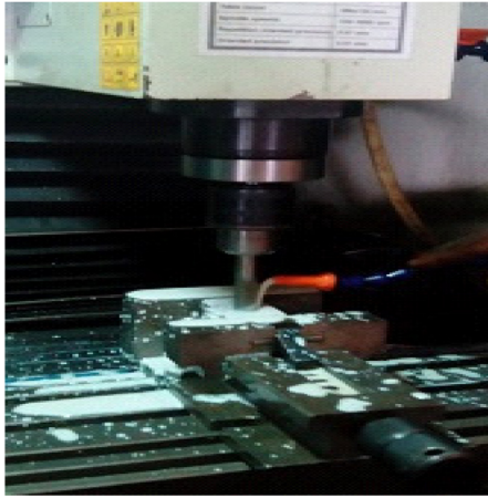
Figure 1. Experimental setup for MQL end milling operation.
