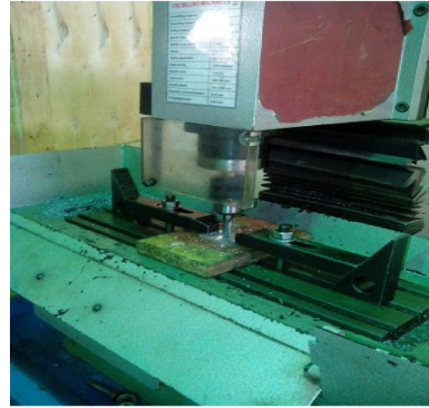
Figure 2. Experimental setup for dry end milling operation.
