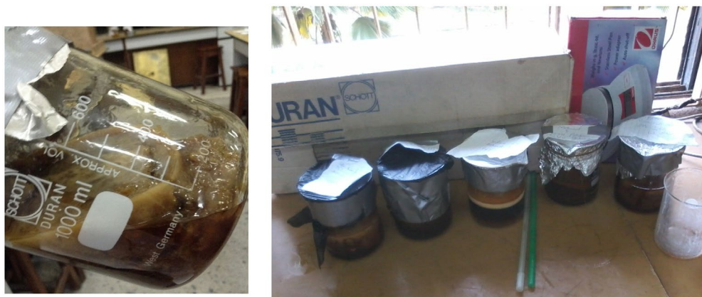
Figure 2. Incomplete production of biodiesel with WVO ethanol using KOH as catalyst.
