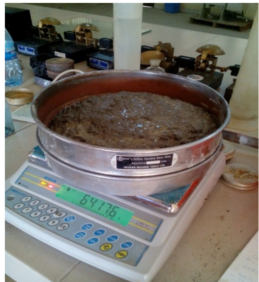
Fig. 4. Segregation resistance test
