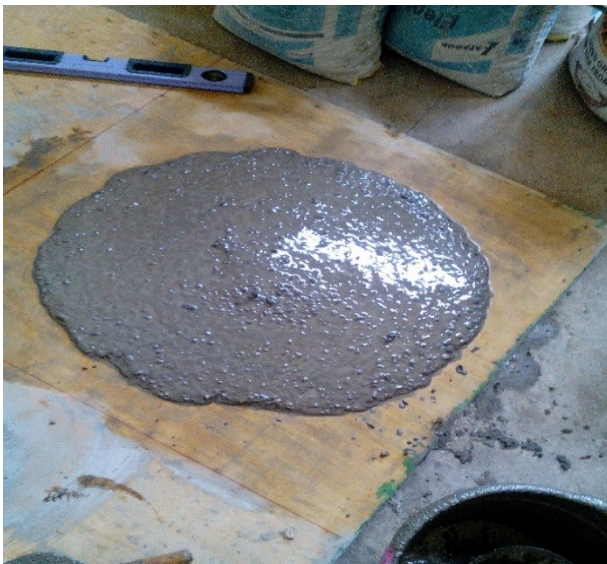
Fig. 3. Slump Flow test
