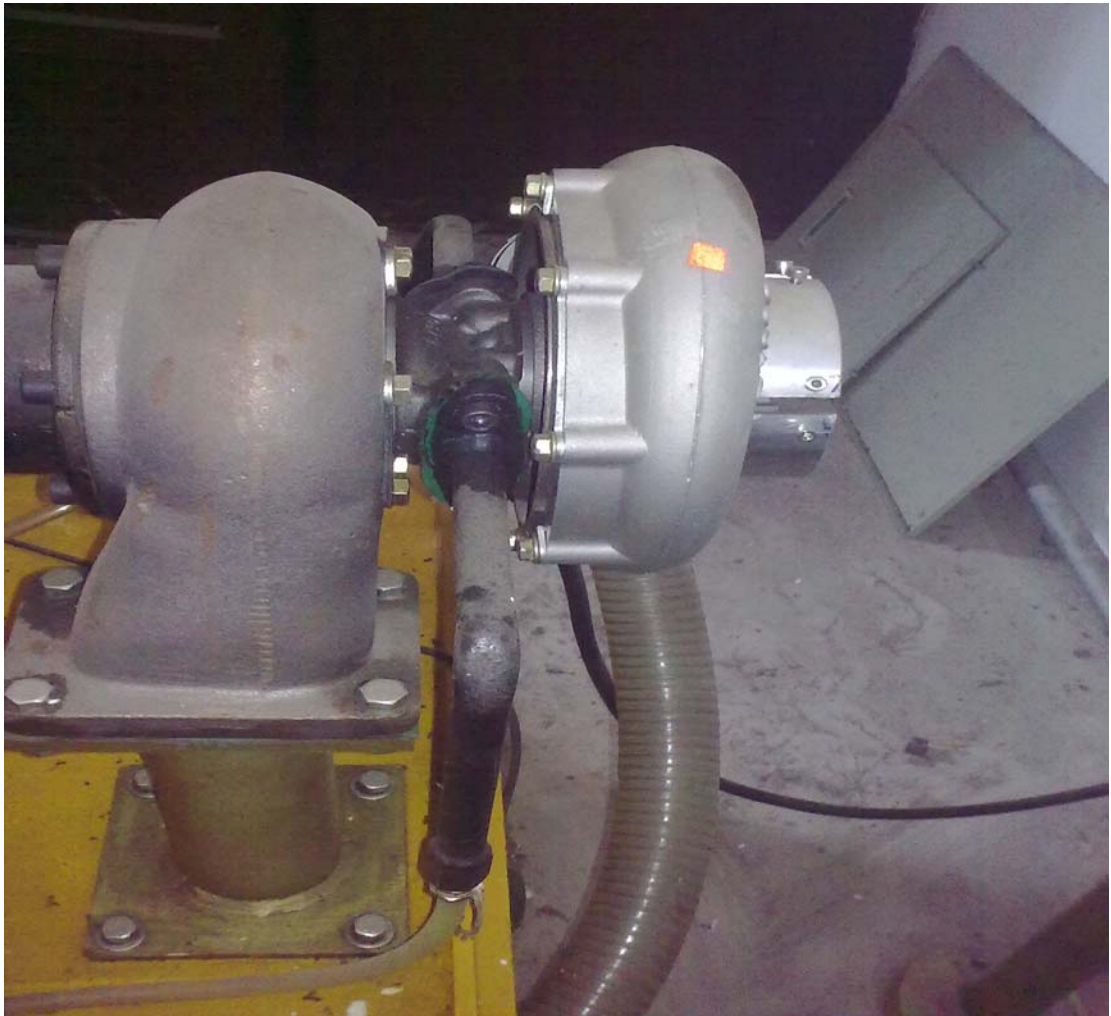
Figure 7. 6. A photograph of the assembly flanges between the lubricant pipe and the turbocharger
