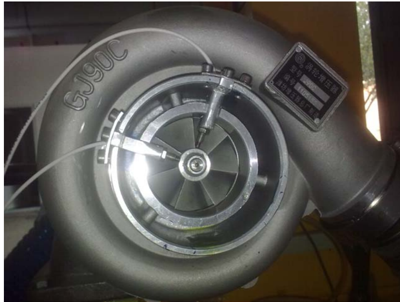
Figure 7. 8. A photograph of the eddy current displacement transducers installed on the turbocharger
