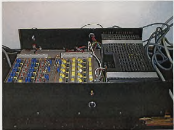
Figure 3. 11 The capacitance measuring system for liquid transport in wound dressings
