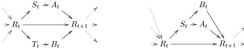
Figure 2: Left: typical perception-action loop of two agents sharing the same environment. R : state of the environment, S, A : sensor and actuator of agent A, respectively T, B for agent B. Right: perception-action loop for a single agent using two distinct actuators A and B .
