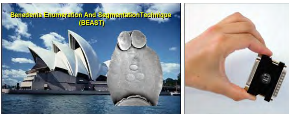
Figure 5. The BEAST program splash page (left). The BEAST macro is accessible through the use of a hardware key or dongle (right) - a plug-in, now via a USB port, which allows the user to access the parent software through which BEAST runs.
