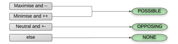
Figure 4.11: Conflict Detection Process of Two Actions for Different Devices
