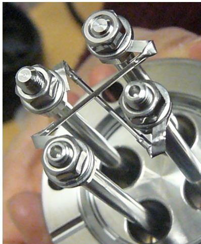
Fig. 7.17: Our rubidium and lithium alkali-metal dispensers (SAES) assembled on the electrical feedthrough.
