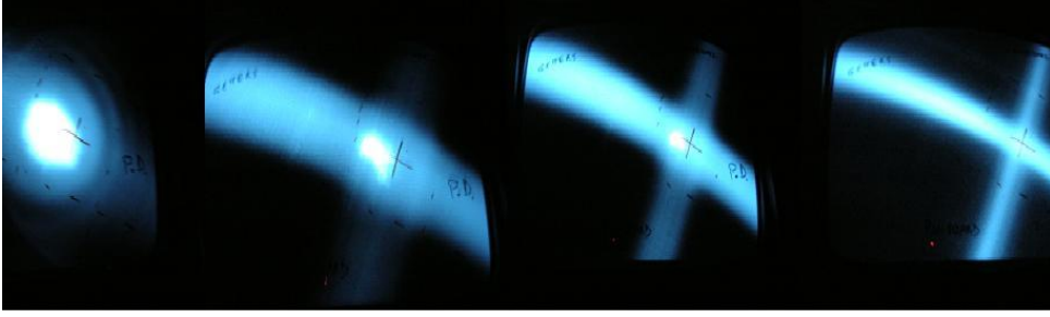
Fig. 4.2: Sequence of images of the MOT beams as the iris is being closed to determine the beam overlap and the beam intersection with respect to the atomic cloud.
