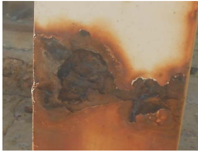
Figure 2. Localized corrosion before the corrosion products have been removed
