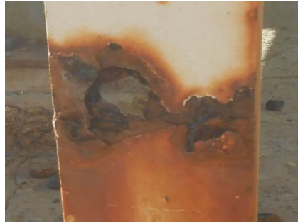
Figure 2. Localized corrosion before the corrosion products have been removed
