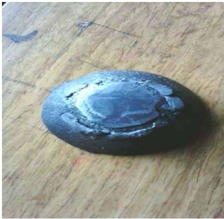
Figure 1: Water quenched sample showing quench cracks
