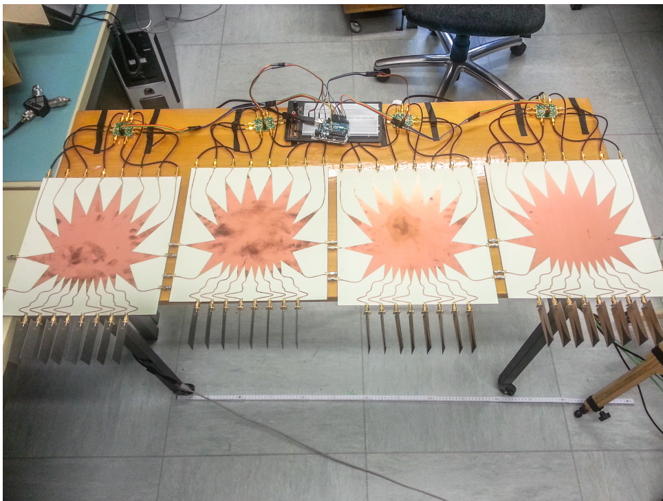
(b) Receiver with Rotman-lens-based hybrid beamforming
