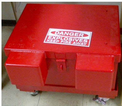
Figure D2: Magazine containing low explosives.
