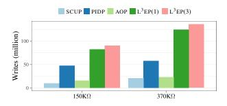
Figure 5.16: The chart shows the expected lifetime of a TLC PCM (in million writes). The *x*-axes group the results by  $\epsilon$ , then by P&V approach.
