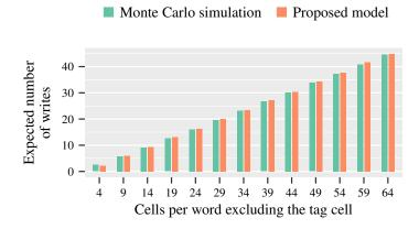
Figure 3.2: The expected number of cell writes using Monte Carlo simulation in comparison to the proposed model (Eq. 3.2).
