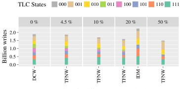
Encodings for different NVM overheads
