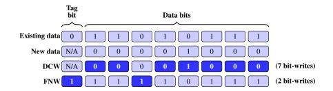
Figure 2.1: For the shown existing and new data, DCW results in 7 bit-writes, whereas FNW, results in only 2 bit-writes. Bit-writes are indicated with darker-color backgrounds.
