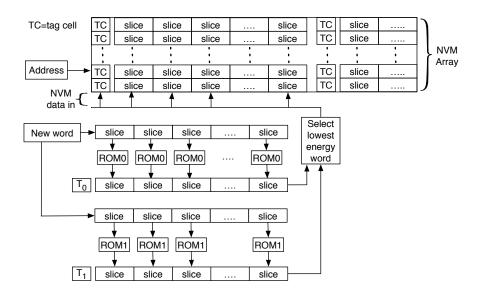
Figure 4.3: An NVM array consists of a number of rows, and each row contains words that are organized as in Fig. 4.1a. An unencoded new word from the CPU is received along with a target address. Then k encoded versions are generated and the word with the lowest energy (with respect to the current word at the target address) is selected for writing. For decoding purposes, each encoded version is associated with a tag value that is stored with the lowest energy version.
