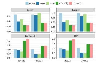
Figure 5.20: This chart shows the energies, latencies, bandwidths, and IPCs of every P&V approach averaged across the workloads in Table 5.4 and normalized to SCUP. This result assumes 16 drivers per memory line for SCUP and 1 driver per memory line for the rest of the P&Vs evaluated.
