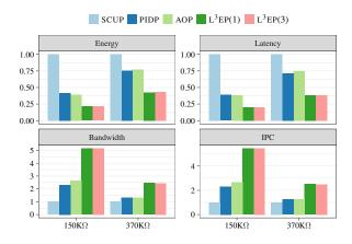
Figure 5.18: This chart shows the energies, latencies, bandwidths, and IPCs of every P&V approach averaged across the workloads in Table 5.4 and normalized to SCUP. This result assumes unlimited write drivers for all the P&Vs evaluated.
