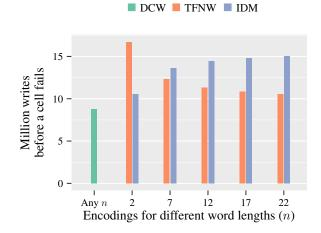
Figure 3.11: The *Y*-axis is the average number of (million) writes per cell before the first cell failure occurs. The *X*-axis lists encoding solutions: TLC DCW, TFNW, and IDM [Niu *et al.* 2013] for different word lengths. Clearly, TFNW performs better for small n. As n gets larger, the endurance effect of TFNW approaches TLC DCW's effect on endurance.
