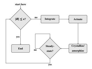
Figure 2.4: In PIDP P&V [Papandreou *et al.* 2011], PIDP examines if  $|E| \leq \epsilon$  and stops if true. Otherwise, it integrates the error signal, converts it into a control command (actuation), and issues either a crystallization or amorphization pulse, depending on the outcome of the actuation. Next, it waits for the steady-state resistance and repeats this process until  $|E| \leq \epsilon$ .
