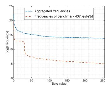
Figure 2.2: In this plot, the x-axis is all the possible values (bytes) and the y-axis is the frequency of the corresponding value in logarithmic scale. Clearly, the frequency profile of benchmark 437.leslie3d exhibits good skew that supports the locality of frequent values. But aggregating the frequency profiles of 32 benchmarks results in a relatively flat plot, suggesting that more than 98% of the values are almost equally likely.
