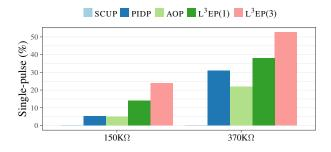
Figure 5.15: The chart shows the percentage of MC iterations in which the programming converges in one pulse. The *x*-axes group the results by  $\epsilon$ , then by P&V approach.
