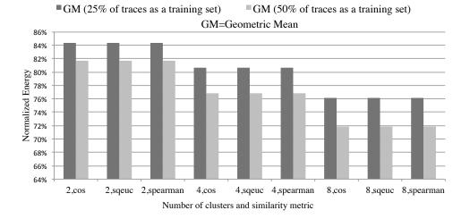
Figure 4.10: TLC case similar to Fig. 4.9. By training on 25% of the applications, write energy increases by only 3.5% on average in comparison to training on 50% of the applications.
