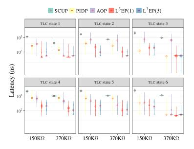
Figure 5.8: Write latencies broken down by TLC state, then by the two write margins, and then by various P&V approaches. The median latencies are indicated by  $\circ$  marks on every violin.
