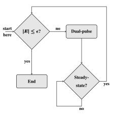
Figure 2.5: In AOP P&V [He *et al.* 2014], AOP examines if  $|E| \le \epsilon$  and stops if true. Otherwise, based on the error, AOP guesses the amplitude of the first dual-pulse using a simple linear model. Next, it waits for the steady-state resistance and repeats this process until  $|E| \le \epsilon$ . Subsequent amplitudes of the dual-pulses are slight increments (or decrements) of the previous amplitude.
