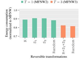
Figure 3.5: The effect of choosing a transform over the other on energy consumption. Here, R,  $S_1$ , and  $S_2$  denote bitwise rotation, swapping MLC states 10 and 11, and swapping MLC states 01 and 11, respectively. All the bars are normalized to MFNW energy consumption.
