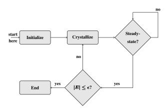
Figure 2.3: In SCUP P&V [Bedeschi *et al.* 2009], SCUP first initializes the cell to the amorphous state. Next, SCUP issues a partial crystallization pulse to slightly lower the resistance, waits for the steady-state resistance, and verifies if the programming error (|E|) is within the write margin ( $\epsilon$ ). If so, SCUP stops, otherwise it repeats the process until the target resistance is reached ( $|E| \le \epsilon$ ).
