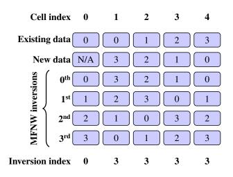
Figure 3.13: Illustration of the inversion index.
