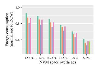
Figure 3.6: Energy consumptions of MFNW, MFNW2, MFNW3, EEE [Wang *et al.* 2011], and TTT [Mirhoseini *et al.* 2015] for different NVM overheads. Energy consumptions are all normalized to DCW energy consumption. While MFNW2 and MFNW3 provides more energy reduction than state-of-the-art encoding solutions for the same NVM overhead, MFNW in its original form can also achieve high energy reductions provided enough NVM overhead.
