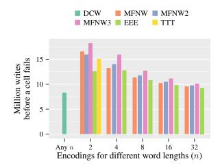
Figure 3.10: The *Y*-axis is the average number of (million) writes per cell before the first cell failure occurs. The *X*-axis lists encoding solutions: MLC DCW, MFNW, MFNW2, MFNW3, EEE [Wang *et al.* 2011], and TTT [Mirhoseini *et al.* 2015] for different word lengths. Clearly, all versions of MFNW perform better for small *n*. As *n* gets larger, the endurance effect of MFNW approaches MLC DCW's effect on endurance.
