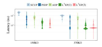
Figure 5.7: Write latencies broken down by the two write margins then by various P&V approaches. The y-axis is in logarithmic scale. The median latencies are indicated by  $\circ$  marks on every violin.
