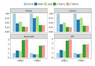
Figure 5.19: This chart shows the energies, latencies, bandwidths, and IPCs of every P&V approach averaged across the workloads in Table 5.4 and normalized to SCUP. This result assumes 16 drivers per memory line for SCUP and 4 drivers per memory line for the rest of the P&Vs evaluated.
