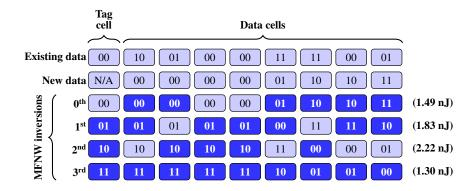
Figure 3.3: For the new and existing data above, CHD MFNW picks the 2<sup>nd</sup> inversion, resulting in minimum cell Hamming distance (but the highest energy too). EHD MFNW picks the 3<sup>rd</sup> inversion, since it results in minimum energy, regardless of cell distance.
