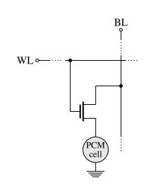
Figure 5.4: A 1T1R PCM cell with an nMOS access device: The PCM cell can be controlled using the bit line (BL) and word line (WL) inputs.
