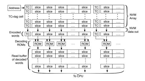
Figure 4.4: Decoding ROMs are replicated for each slice across the memory line. ROMs are addressed by slice value augmented with tag value.
