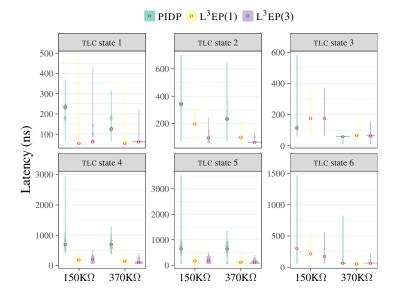
Figure 5.9: Similar to Fig. 5.8, but compares PIDP,  $L^3EP(1)$ , and  $L^3EP(3)$ . Also, the *y*-axis is linearly scaled in this figure. The median latencies are indicated by  $\circ$  marks on every violin.
