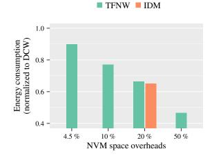
Figure 3.8: Energy consumptions of TFNW (for different NVM overheads) and IDM [Niu *et al.* 2013]. For the same NVM overhead as IDM, TFNW achieves almost the same geometric mean energy reduction. When NVM overhead is relaxed to 50%, TFNW can achieve more than 53% energy reduction. Energy consumptions are all normalized to DCW energy consumption.
