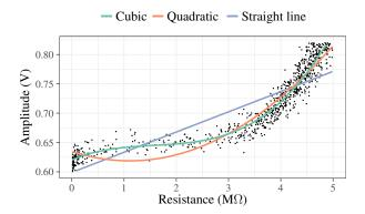
Figure 5.5: Regression plot of the steady-state PCM cell resistance (x-axis) versus the amplitude of the first amorphization pulse (y-axis). The scatter graph is the regression dataset. Linear, quadratic, and cubic models are shown. We assume a 32 nm PCM cell and access device with parameters from Table 5.2.
