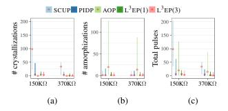
Figure 5.13: These plots show the number of (a) crystallization, (b) amorphization, and (c) total pulses of the 60K MC iterations broken down by the two write margins and then by various P&V approaches.
