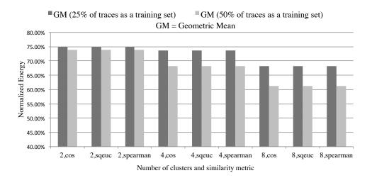
Figure 4.9: Geometric mean (GM) of MLC write energies, normalized to DCW. The two cases are training on 50% of the applications and evaluation on 50% versus training on 25% and evaluation on 75%. By training on 25% of the applications, write energy increases by only 3.34% on average.
