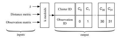
Figure 4.2: Given the number of clusters k, the required similarity metric, and the observation matrix, the k-medoids algorithm divides the 32 observations (applications) into k clusters ( $0 \le C_i < k$  and  $0 \le i < 32$ , where  $C_i$  is the cluster ID of observation i.)
