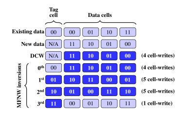
Figure 3.1: For the shown existing and new data, DCW results in 4 cell writes. CHD MFNW chooses to write the 3<sup>rd</sup> inversion of the new data, since it results in the minimum number of cell writes (1) among all other inversions. Note that cell-writes are indicated with darker-color backgrounds.
