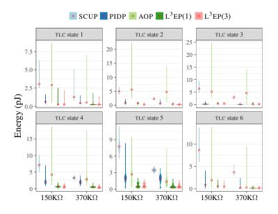
Figure 5.11: Write energies broken down by TLC state, then by the two write margins, and then by various P&V approaches. The median energies are indicated by  $\circ$  marks on every violin.
