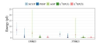
Figure 5.10: Write energies broken down by the two write margins then by various P&V approaches. The median energies are indicated by  $\circ$  marks on every violin.
