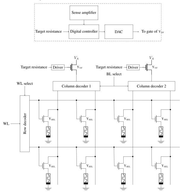
Figure 5.21: This example illustrates how to setup multiple  $L^3EP$  drivers. The voltage-follower nMOS (VF) is assumed to be strong enough to drive one bit line. The internals of the "driver" block are shown in the subfigure surrounded by a dashed rectangle. It consists of a digital-to-analog converter (DAC), and a sample–and–hold (S/H) circuit. The output of the S/H circuit is connected to the gate terminal of the VF.
