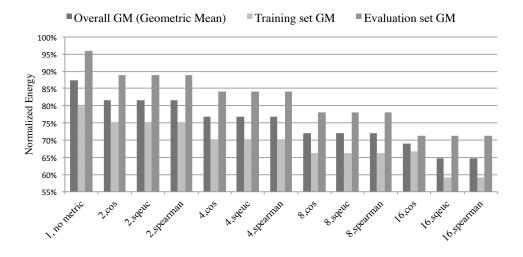
Figure 4.8: Results for TLC RRAM, organized similar to Fig. 4.6. The gap between write energies of the training and evaluation sets consistently decreases as k increases, except for the case from k = 8 to k = 16 for the square Euclidean and Spearman metrics (12% in both cases).
