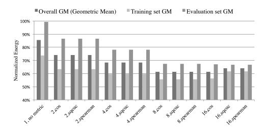
Figure 4.6: Each group of three bars represent the overall geometric mean (GM), training set GM, and evaluation set GM of MLC write energies. Similar to Fig. 4.5, write energies are normalized to DCW. As the number of clusters increases, the gap between write energies of the training set and evaluation set reduces.
