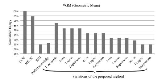
Figure 4.7: Results, organized similar to Fig. 4.5, for state-of-the-art TLC encoding solutions (left to right): MFNW for TLC, incomplete data mapping (IDM) [Niu *et al.* 2013], and perfect knowledge FVE. Again, write energies are normalized to DCW.
