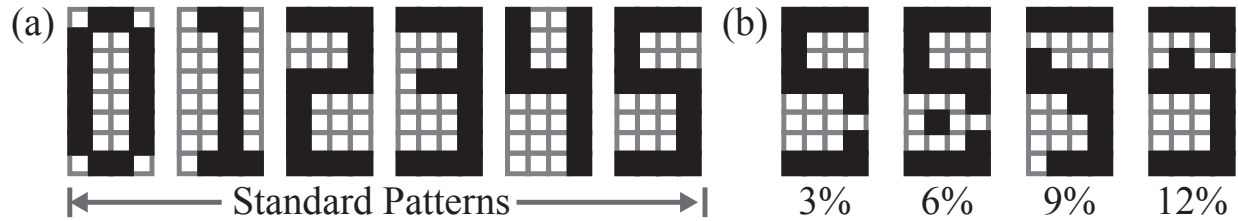
Figure 19: (a) The standard training set of six patterns. (b) An example of noise pattern “5” under different single bit error rate.
